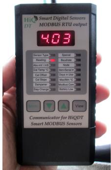
Handheld Communicator (HHC) has 3-digit display & 16 LEDs to show analytic data & readings as well as to calibrate & configure sensor. Programming is done with 4 keys. 'Mode' key toggles & navigate to each LED. 'Up' or 'Down' buttons scroll options & adjust values. 'Mode' key makes selections & saves entries. 'View' key used to provide additional information for the given LED mode (see manual for specifics in each LED).
