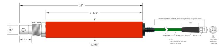
Drawing for K = 0.05, 0.10, 0.20, 0.50, 1.0 & 2.0 /cm cells. Longer 2.25" insertion depth is available with 11.3" overall length.
