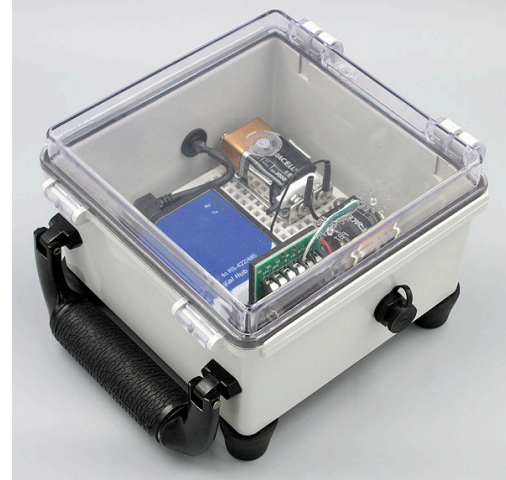
Portable HiQ to Windows Bridge Box with industrial RS-485 to USB converter. Top angle view showing rugged carrying handle & rubber feet. Sealing caps ensure NEMA4X rating when sensor input and USB output ports are not in use.
