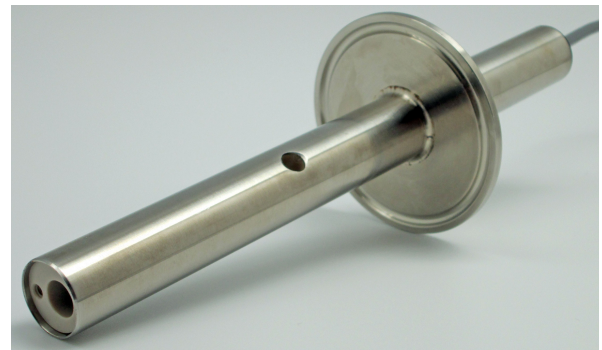
K=5.0/cm configuration has the vent hole location 3.0 inches from the tip of the sensor. As shown in this configuration the flange to tip length is 5.0 inches (min is 4.0 and max is 7.0). The K=5.0/cm cell constant configuration can measure up to 500mS/cm when interfaced with a suitable mating transmitter.
