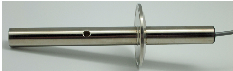
K=2.0/cm cell constant configuration has vent hole and inner electrode just 03 inches from tip. The distance from flange to tip is 3.0 inches with an overall length of 5.0 inches. The K=2.0/cm cell constant configuration can be used to measure conductivity up to 200mS/cm with a suitable mating transmitter.
