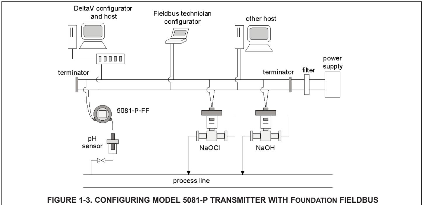
FIGURE 1-3. CONFIGURING MODEL 5081-P TRANSMITTER WITH FOUNDATION FIELDBUS
