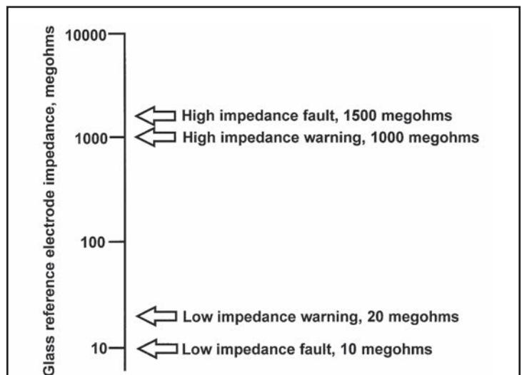
**FIGURE 10-2. Suggested Glass Impedance Warning and Failure Limits for a Glass Reference Electrode**
