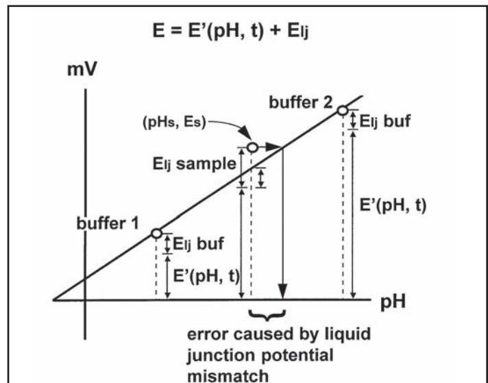
**FIGURE 13-8. Liquid Junction Potential Mismatch.**
