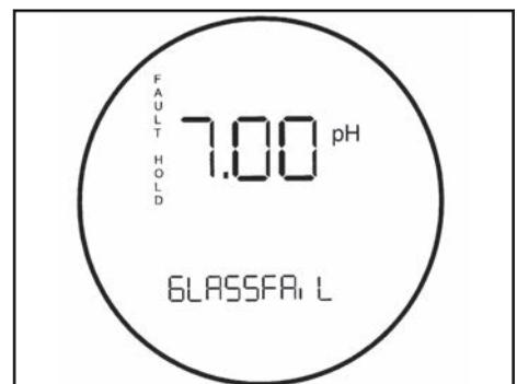
**FIGURE 12-2. Fault Annunciation**
