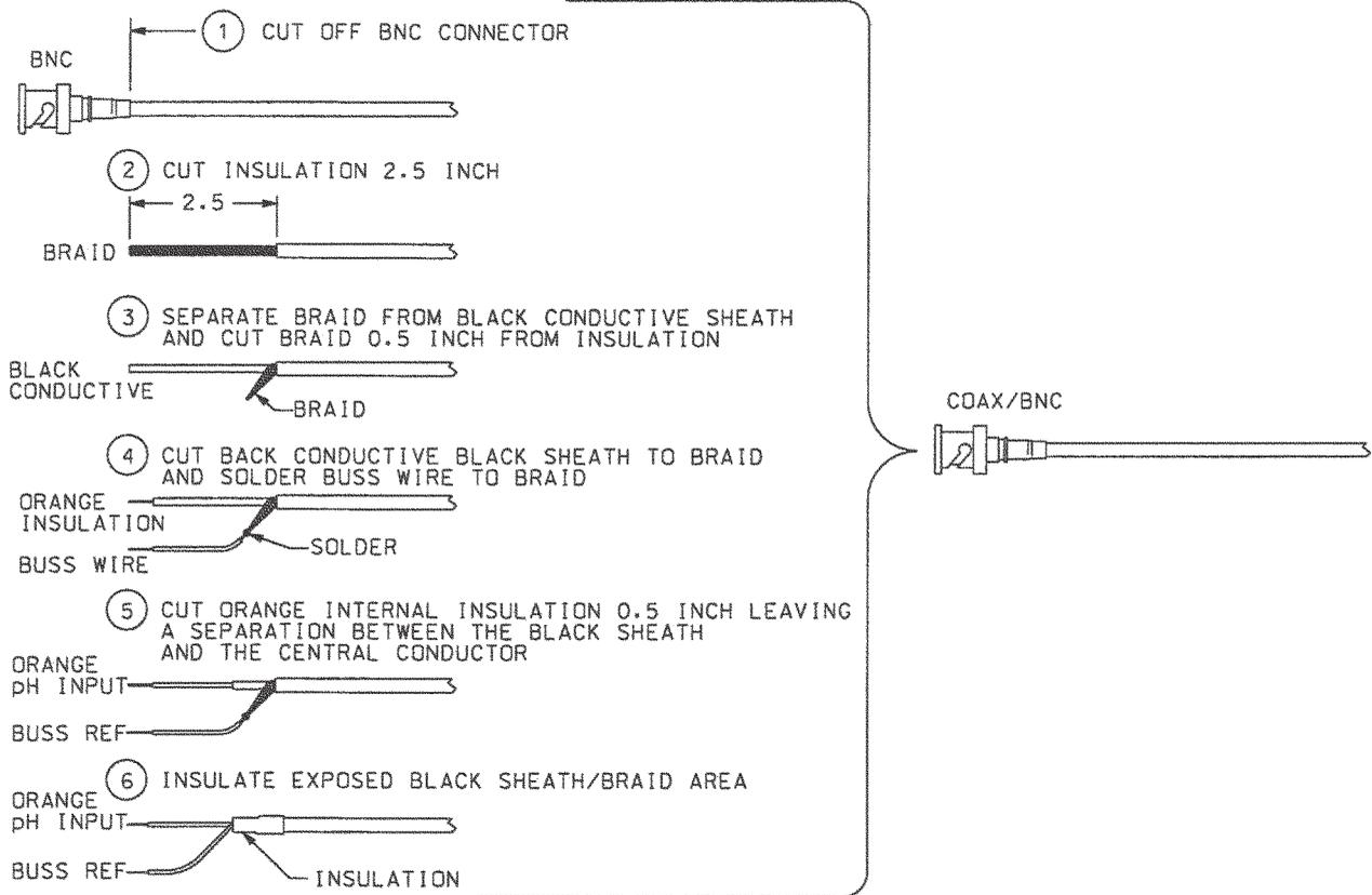
FIGURE 3-20. Procedure for Removing BNC Connector and Preparing Coaxial Cable
