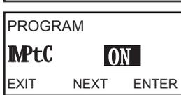
5. The **IMPtC** prompt appears. Use the **↑** or **↓** keys to enable (**On**) or disable (**OFF**) glass impedance temperature compensation. Because glass impedance is a strong function of temperature, correcting glass impedance for temperature is recommended. A third setting (**SPC**) appears in addition to **On** and **OFF**. Do not select **SPC**; the setting is intended for factory use. Press ENTER to save.
