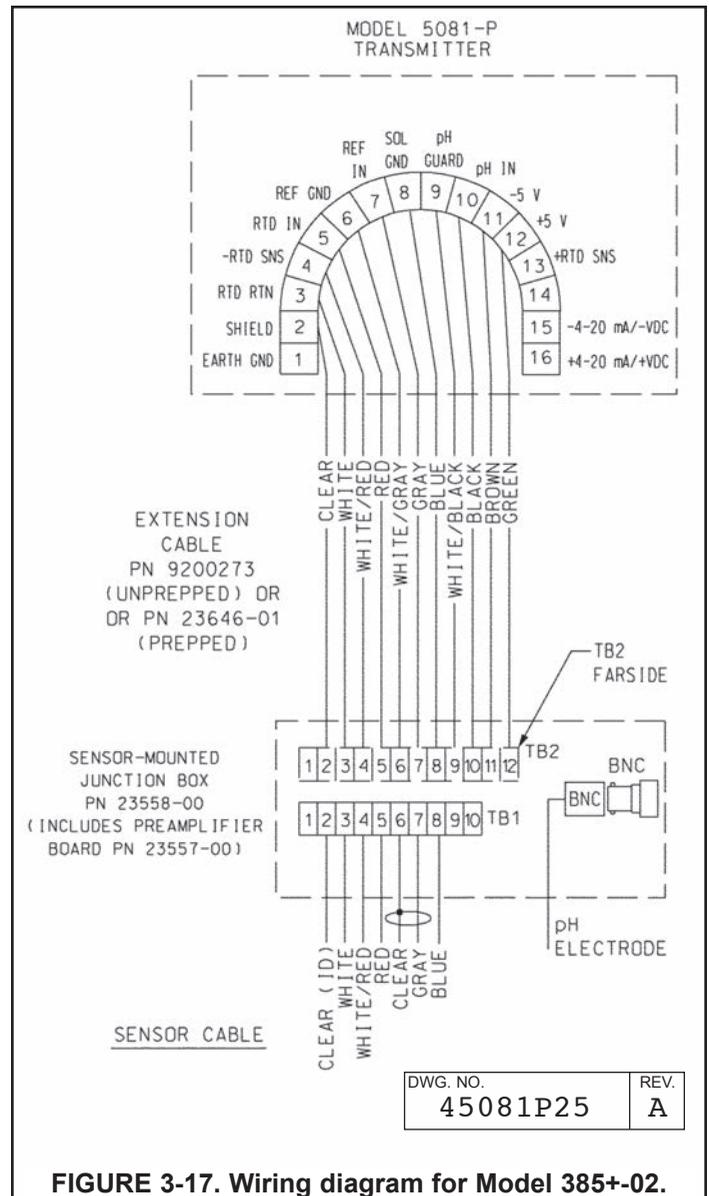
FIGURE 3-17. Wiring diagram for Model 385+02.
