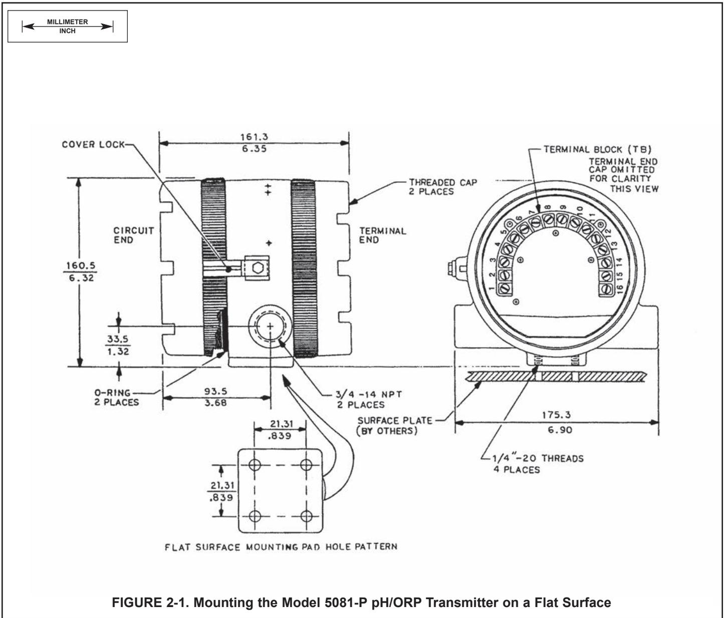
FIGURE 2-1. Mounting the Model 5081-P pH/ORP Transmitter on a Flat Surface
