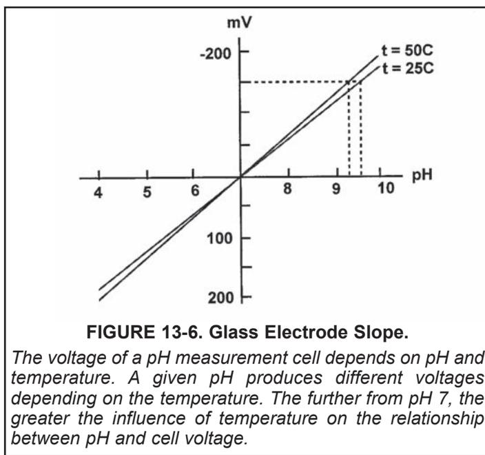
The slope of the isotherm is often called the glass electrode or sensor slope. The slope can be calculated from the equation:  $\text{slope} = 0.1984 (t + 273.15)$ , where  $t$  is temperature in  $^\circ\text{C}$ . The slope has units of mV per unit change in pH. The table lists slopes for different temperatures.
