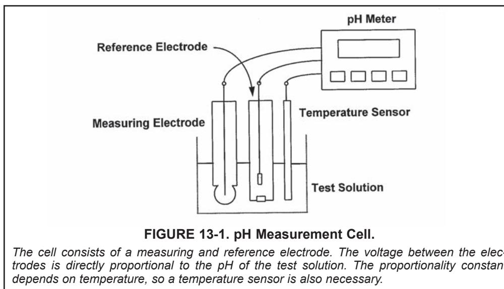
Figure 13-1 shows separate measuring and reference electrodes. In most process sensors, the electrodes and the temperature element are combined into a single body. Such sensors are often called combination electrodes.
