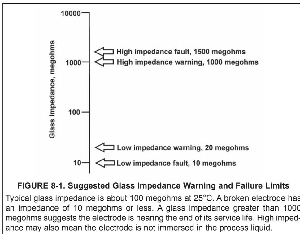
4. REFERENCE IMPEDANCE. The majority of reference electrodes used in industry are low impedance silver-silver chloride electrodes. Every pH and ORP sensor manufactured by Rosemount Analytical has a low impedance reference. However, there are applications that call for either a high impedance sodium or pH glass reference electrode. Both high impedance and low impedance reference electrodes can be used with the Model 5081-P pH/ORP transmitter.
