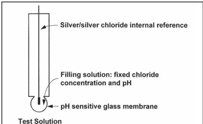
**FIGURE 13-2. Measuring Electrode.**
