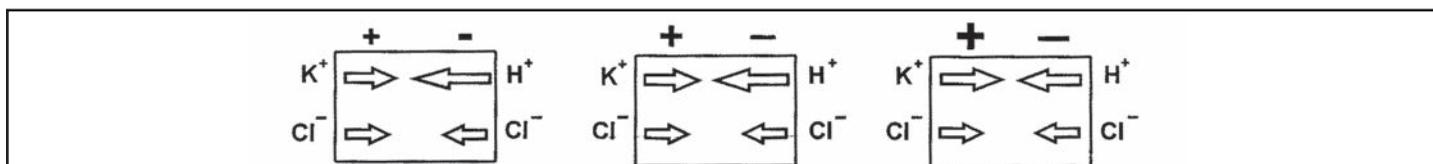
**FIGURE 13-5. The Origin of Liquid Junction Potentials.**
