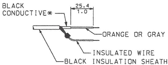
\* WARNING: IF INNER BLACK CONDUCTIVE SHEATH IS IN CONTACT WITH THE EXPOSED LEADS, OR IS NOT PREPARED PROPERLY, IT MAY CAUSE AN ELECTRICAL SHORT.
