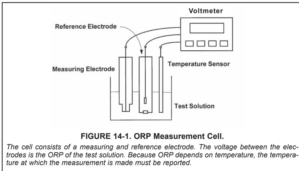
Figure 14-1 shows separate measuring and reference electrodes. In most process sensors the electrodes and the temperature element are combined into a single body. Such sensors are often called combination electrodes.
