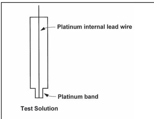
**FIGURE 14-2. Measuring Electrode.**
