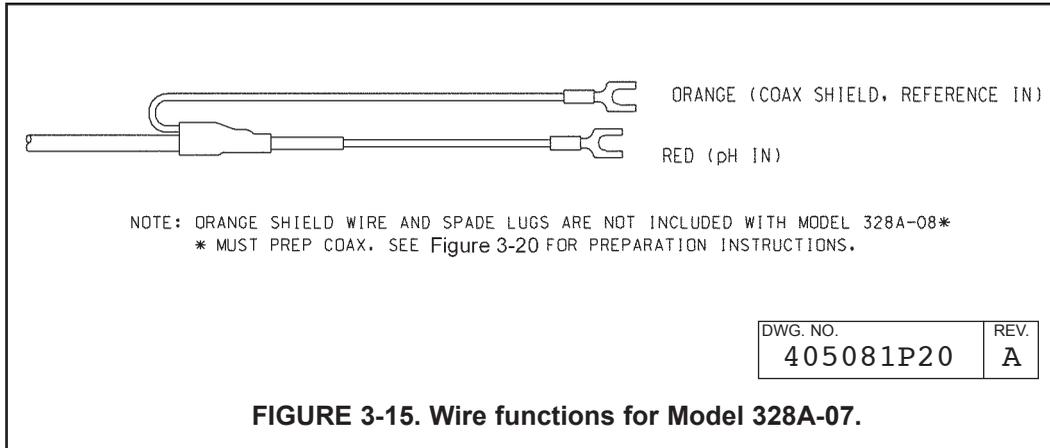
FIGURE 3-15. Wire functions for Model 328A-07.
