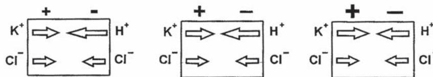
**FIGURE 14-4. The Origin of Liquid Junction Potentials.**
