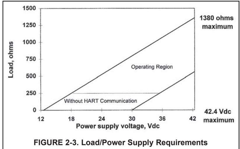
FIGURE 2-3. Load/Power Supply Requirements
