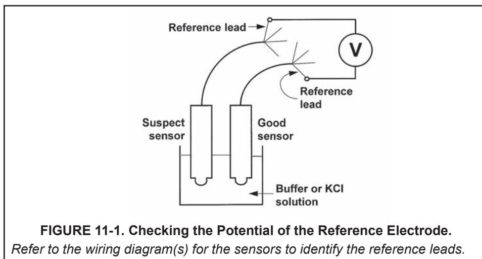
A laboratory silver/silver chloride reference electrode can be used in place of the second sensor. All Rosemount Analytical pH sensors have a silver/silver chloride reference, and most sensors use gelled saturated potassium chloride for the fill. The potentials of a good sensor reference electrode and a saturated silver/silver chloride laboratory electrode will agree within about 20 mV.
