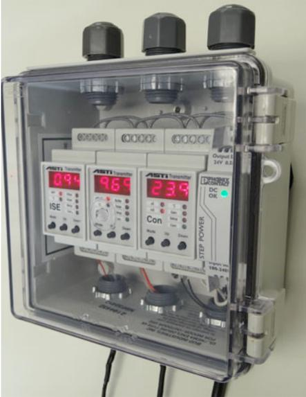
*Triple Channel Nitrate, pH & Conductivity Transmitter
