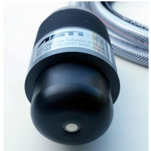
*Close-Up of the fully submersible AST-DO-T Galvanic DO sensor with Pt100 TC is above.*
