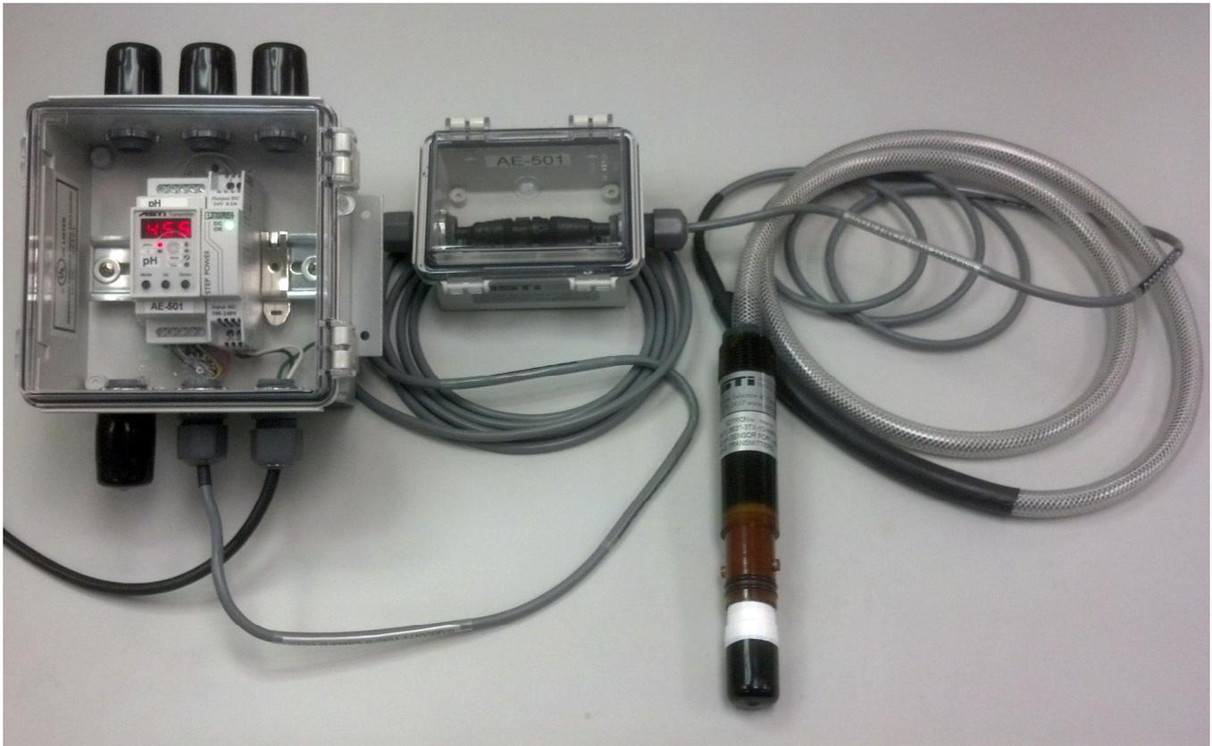
The Q5M (male) quick disconnect termination from the sensor are mated to the Q5F (female) quick disconnect termination for the cable extension inside the 1MF NEMA 4X waterproof J-Box. The sealing cable glands must be well secured to both the 1MF enclosure as well as onto the cables, and the lid must be fastened shut to preserve the NEMA 4X rating.
