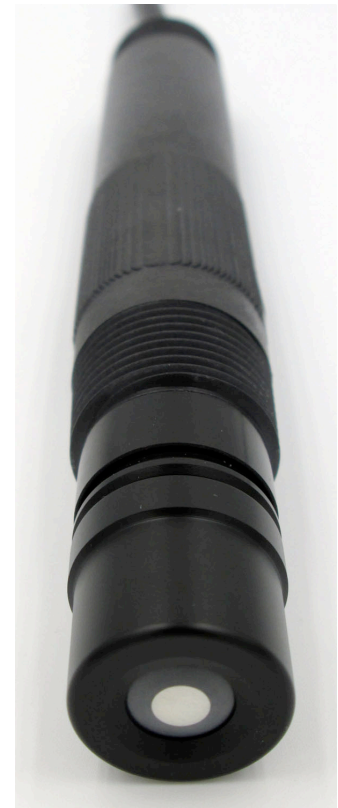
AST-DO-UNIVERSAL dissolved oxygen sensor in convertible configuration; Close-up on DO cell
