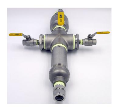
1. Real-Time Monitoring of Critical Parameters In industrial manufacturing, monitoring parameters such as pH, ORP, and temperature is essential to ensure that chemical reactions and biological processes occur within the specified ranges. HOT-TAP Valve Retractable Assemblies allow sensors to be inserted directly into the process stream, providing real-time data without the need to halt production.
