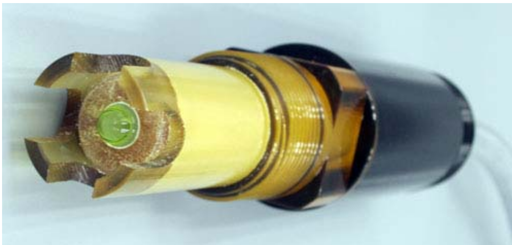
Front View of ZEUS™ pH Sensor Sensing Tip
