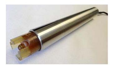
5731 Aggressive Dissolved Gas & Solvent Resistant pH sensor Close-up view of tip with 4 each "GR" thick protective tines Double sealing 0-rings for integrity & safety of installation Ideal for organic manufacturing processes employing volatile solvents& pressurized vessels requiring safe HOT-TAP use Standard Viton®-75 0-rings with CV75, Simriz® 485 & Kalrez® 4079 optional as required
