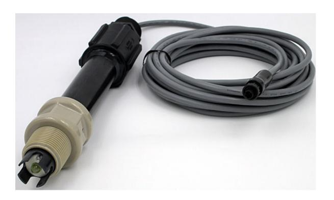
Replacement pH & ORP Sensors For Transmitters that support and/or require Integrated Preamplifiers
