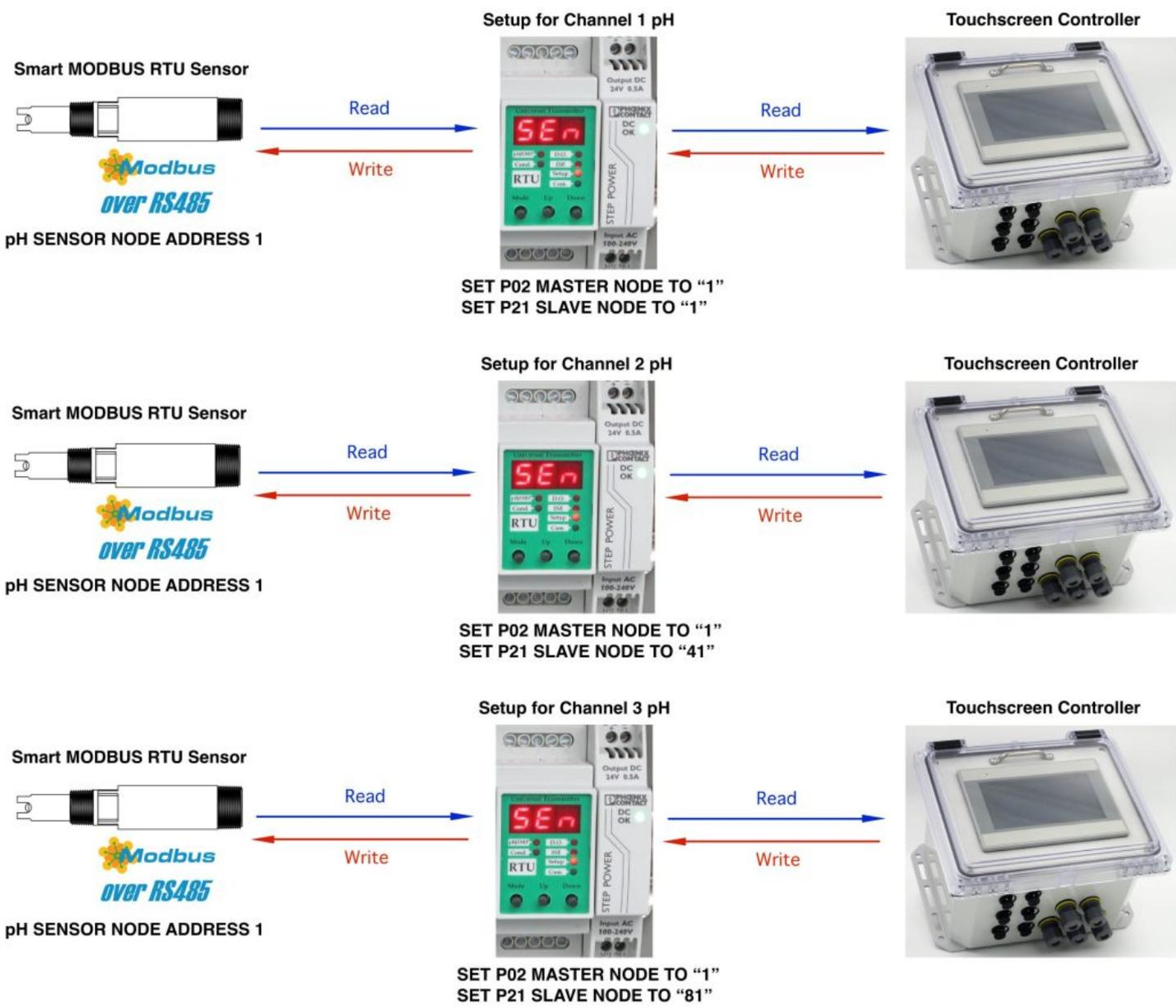
Example shown above is for use with touchscreen controller where channels 1, 2 & 3 are configured for pH. This scheme allows for seamless hot-swap plug and play operation without having to change the node address on the smart pH sensor no matter the channel. The 3TX-RTU-D P21 slave node address defines the channel to the touchscreen controller to which it is connected. For other sensor types the P02 and P21 node address assignments would differ but the concepts would be the exactly the same as
