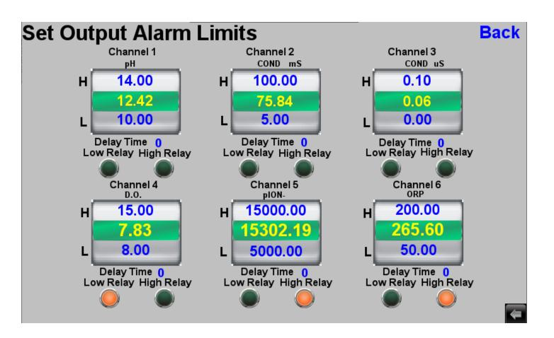
High & Low relay process setpoints for each channel with time delay.
