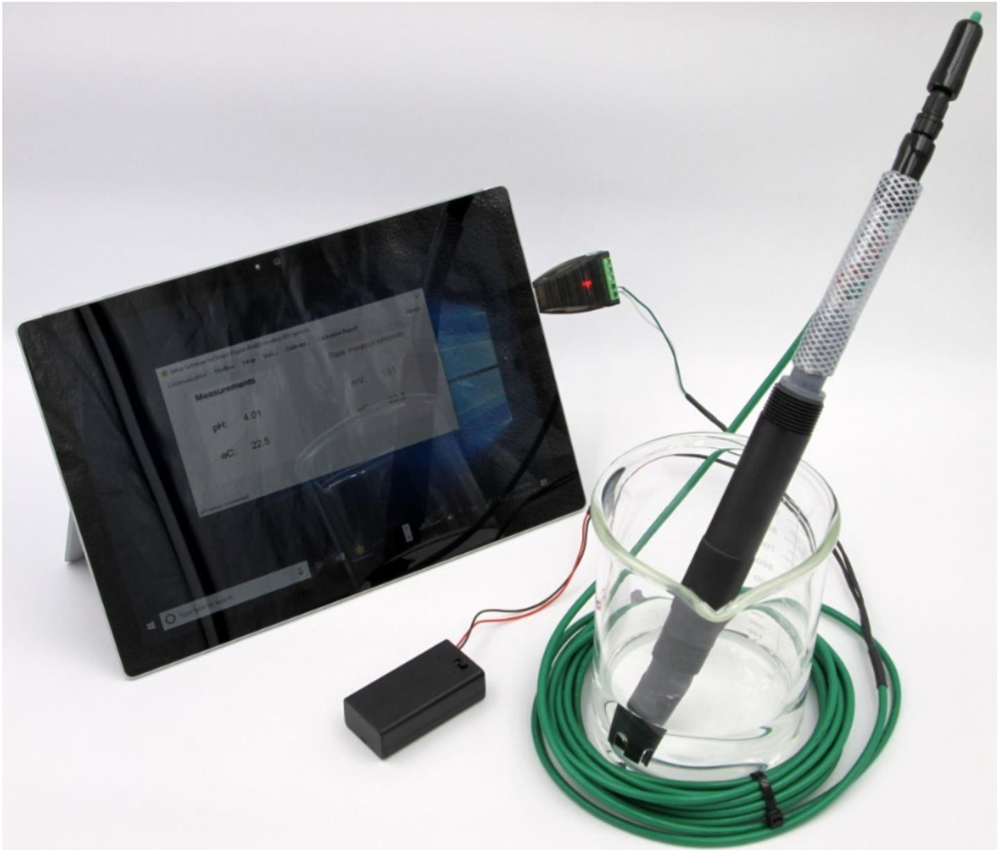
*Low-cost battery-powered bridge assembly to power smart digital HiQDT MODBUS RTU sensors and RS-485 to USB converter to interface with Windows software on PC or surfacet tablet touchscreen.*
