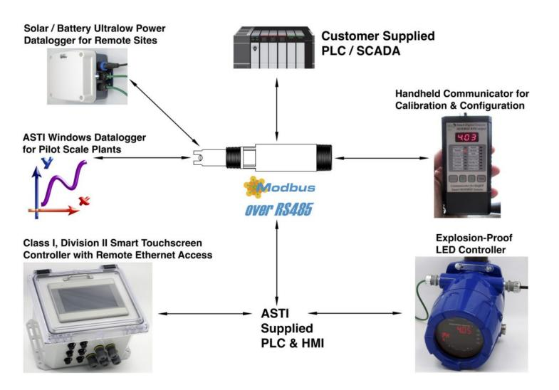
The HiQDT product line is designed to allow for seamless integration with either customer supplied PLC & HMI or else available as turn-key plug and play packages from the ASTI factory ready for commissioning right out of the box. Systems are available for continuous inline measurement and control in hazardous or safe locations employing rugged LED or advanced touchscreen interfaces.
