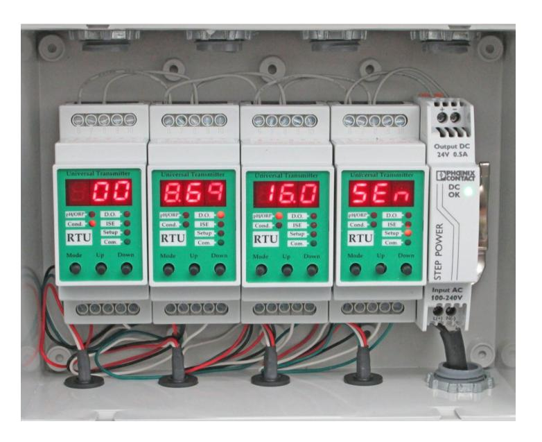
• Type of connected sensor is indicated with illuminated LED in main display mode. If node of sensor is not known the automated search node feature will find it. Once the node address is found the sensor type is automatically determined.
