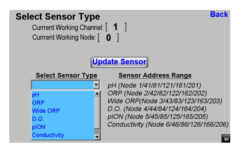
Measurement type for each channel on universal controller assigned or modified at any time using smart digital hot-swap plug & play sensors.
