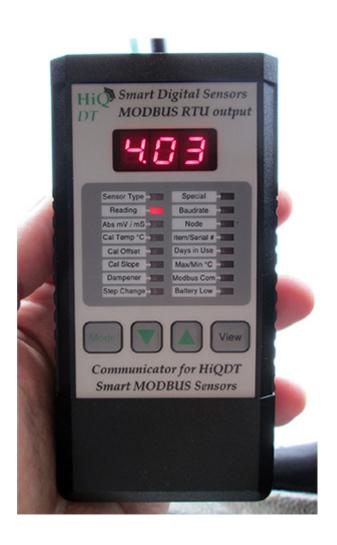
Handheld Communicator (HHC) has 3-digit display & 16 LEDs to show analytic data & readings as well as to calibrate & configure sensor. Programming is done with 4 keys. 'Mode' key toggles & navigate to each LED. 'Up' or 'Down' buttons scroll options & adjust values. 'Mode' key makes selections & saves entries. 'View' key used to provide additional information for the given LED mode (see manual for specifics in each LED).
