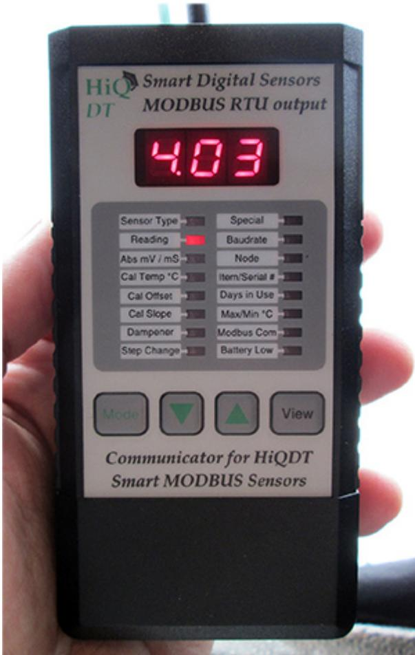
*Handheld Communicator (HHC) has 3-digit display & 16 LEDs to show analytic data & readings as well as to calibrate & configure sensor. Programming is done with 4 keys. 'Mode' key toggles & navigate to each LED. 'Up' or 'Down' buttons scroll options & adjust values. 'Mode' key makes selections & saves entries. 'View' key used to provide additional information for the given LED mode (see manual for specifics in each LED).*
