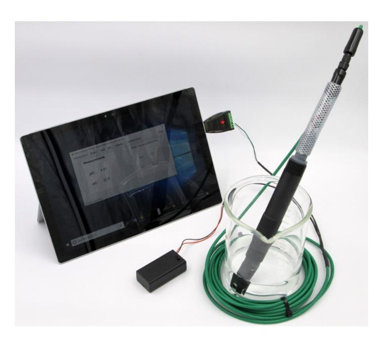
Low-cost battery-powered bridge assembly to power smart digital HiQDT MODBUS RTU sensors and RS-485 to USB converter to interface with Windows software on PC or surfacet tablet touchscreen.
