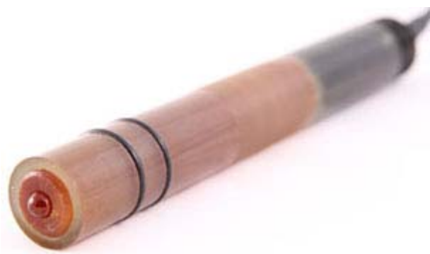
Model 5331 RADEL bodied sanitary pH sensor shown with low-profile break-resistant parabolic pH glass element for use in high viscosity and slurry abrasives type solutions in the without protective tines configuration
