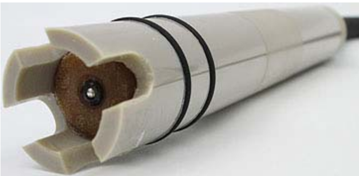
Model 5841 PEEK bodied sanitary ORP sensor shown with low-profile ball-style platinum ORP sensing element for use in high viscosity and slurry abrasives type solutions in the with 4 each "GR" protective tines configuration
