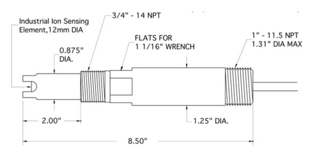
1"-1.25" MNPT IMMERSION & SUBMERSIBLE SERIES SENSORS DIMENSIONAL DRAWINGS
