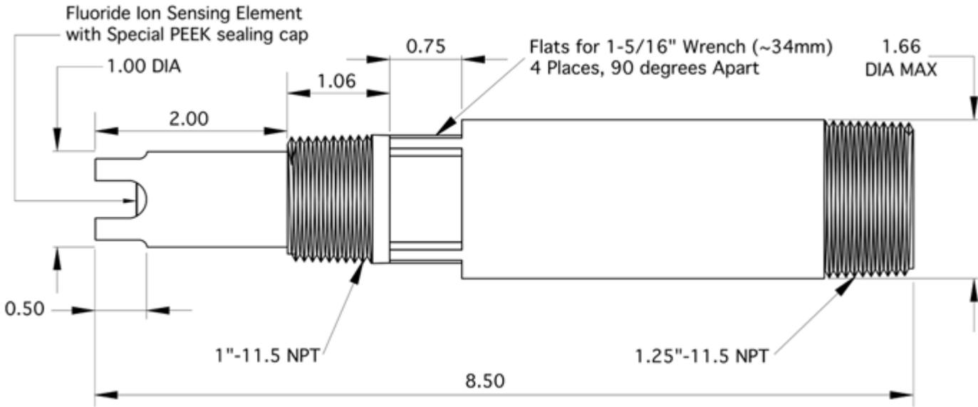
**3/4" MNPT SANITARY & HOT-TAP STYLE SERIES SENSORS DIMENSIONAL DRAWINGS**
