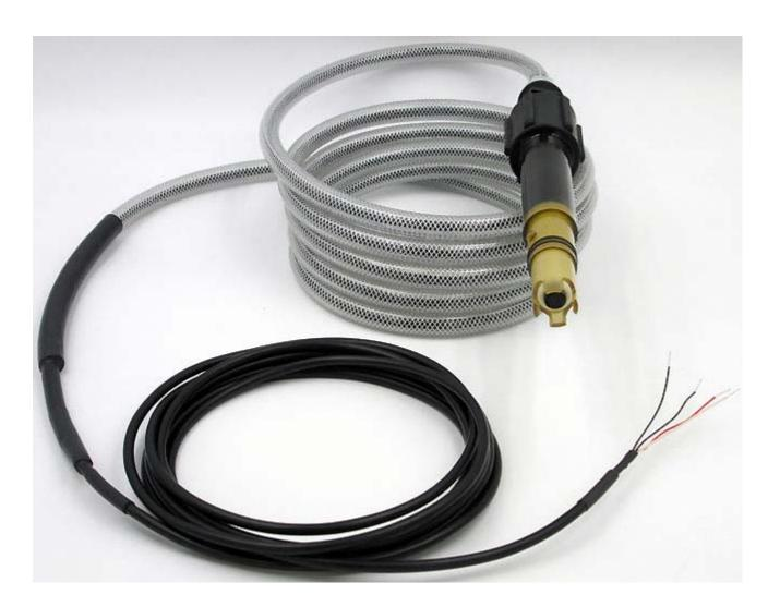
**Calcium** (Ca<sup>2+</sup>) ion selective sensors for determined of ionized free unbound calcium levels to determine the state of the water softeners to automate regeneration as well as a proxy for the total water hardness.
