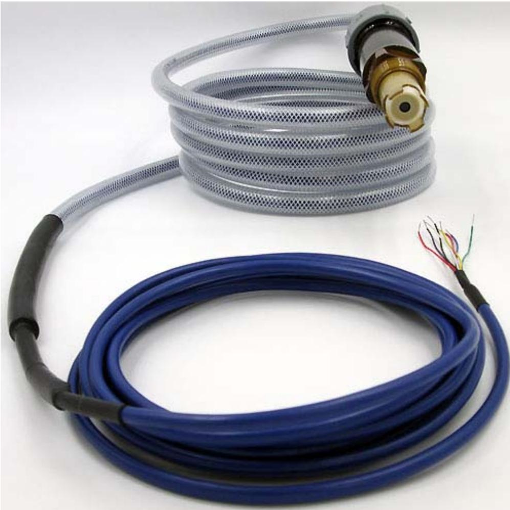
***AB 6100 Fluoride Ion Selective ISE sensor for Acid Service and Fluoride WWT applications; Integral Preamplifier with Braid Reinforced Blue Cable; Fully submersible assembly with waterproofing sealing option "H"***
