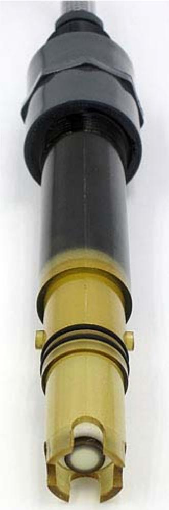
*\* ABGR 8410 Ammonium ISE Sensor available in standard & ultra-low type membrane configurations*
