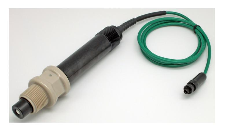
AST-DO-UNIVERSAL-CONVERTIBLE-HiQDT-WPC Smart Digital HiQDT RS-485 MODBUS RTU dissolved oxygen sensor is ready for immediate field installation into  $\frac{3}{4}$ " FNPT process connection for inline use and  $\frac{3}{4}$ " NPT immersion rod or standpipe for fully submersible use.
