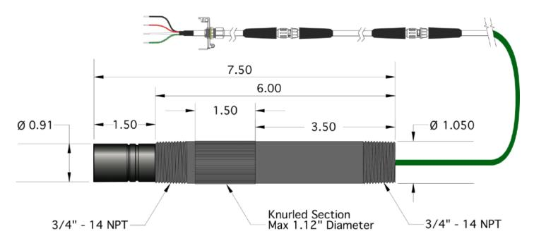
The AST-DO-UNIVERSAL smart digital MODBUS RTU dissolved oxygen sensor is a robust industrial grade sensor measures the dissolved oxygen ppm and percent (%) saturation values including salinity correction. The probe is very rugged and easy to use with automated dry in air smart calibration suitable for use in the toughest industrial, municipal, environmental and aquaculture applications.
