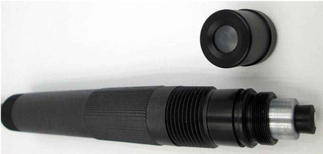
*Close-Up on galvanic DO measuring cell of dissolved oxygen sensor in convertible configuration in fully assembled state ready to use.*
