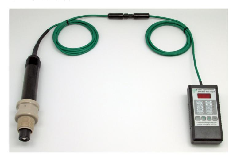
Handheld Communicator and Smart Digital D.O. sensor connection is waterproof NEMA 6P
