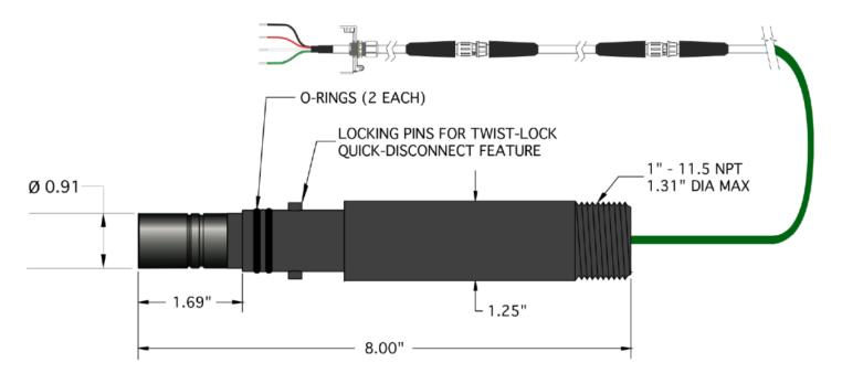
Drawing shown above in the standard inch insertion depth of 0.70 inches past start of  $1\,^{\prime\prime}$  MNPT threads on twist lock receptacle.
