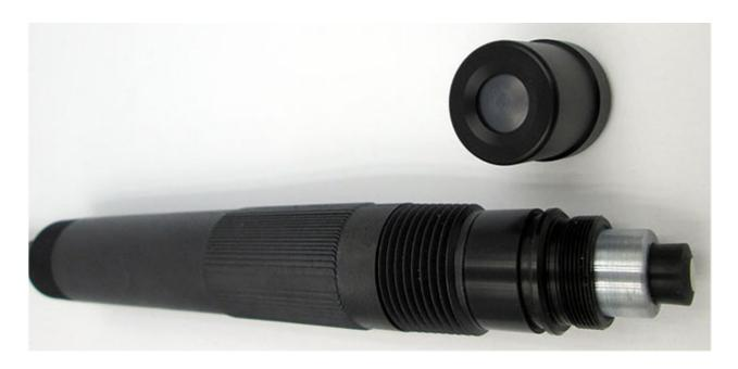
Close-Up on galvanic DO measuring cell of dissolved oxygen sensor in convertible configuration in fully assembled state ready to use.
