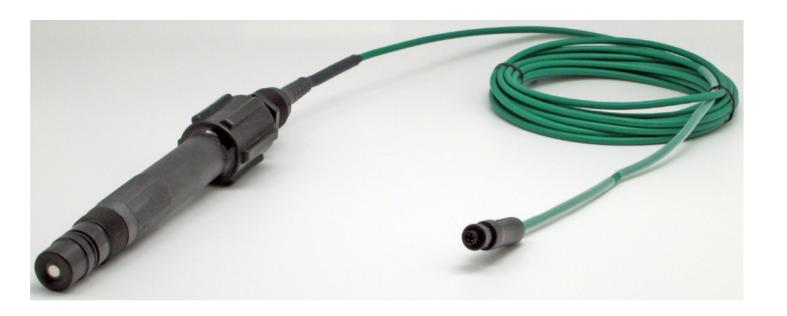
Twist Lock Style Smart Digital HiQDT MODBUS RTU dissolved oxygen sensors interface 1"MNPT Twist Lock Receptacle for quick disconnect bayonet style insertion and removal from process line for ease of removal for cleaning and recalibration which is ideal for inline installations.
