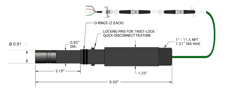
Drawing shown above in the extended inch insertion depth of 2.20 inches past start of  $1^{\prime\prime}$  MNPT threads on twist lock receptacle.
