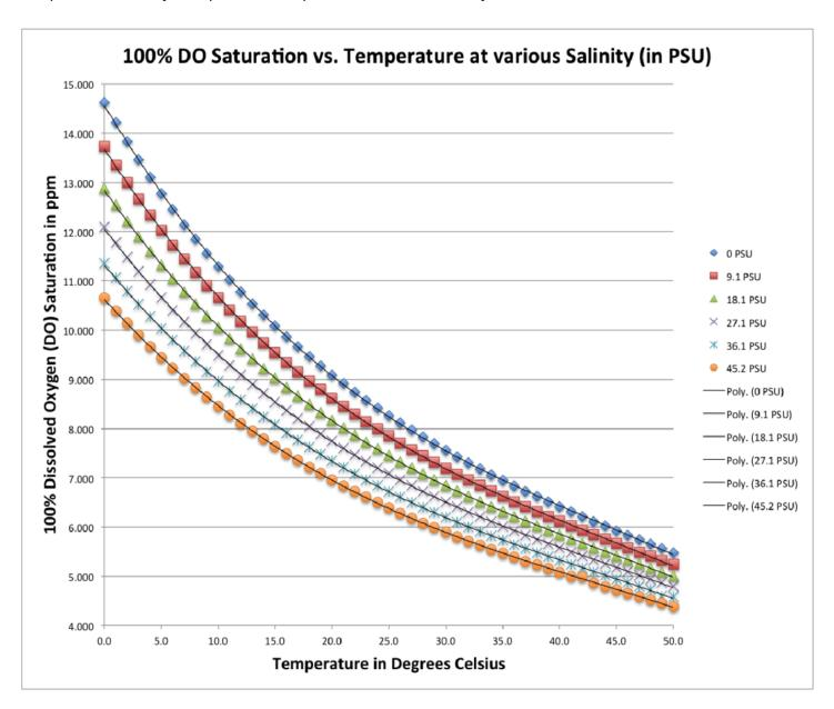
This salinity correction is only required as a correction to the computation of the %
