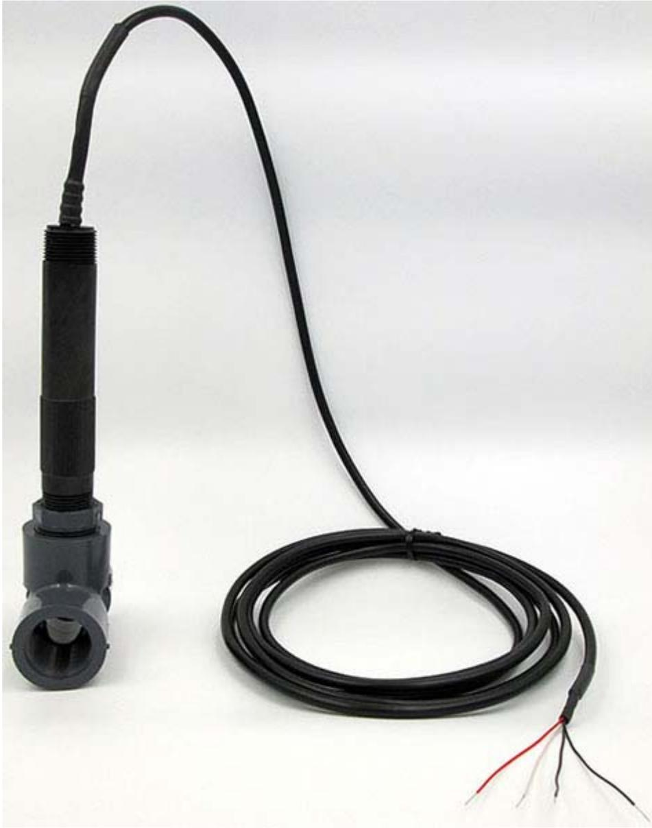
*AST-DO-UNIVERSAL dissolved oxygen convertible style galvanic DO sensor shown threaded into tee with front 3/4" MNPT threads for inline use. Alternate inline installation scheme is using the 1" MNPT twist lock quick disconnect bayonet style hardware setup to allow for fast and simple removal & installation from process without damaging the cable due to coiling.*
