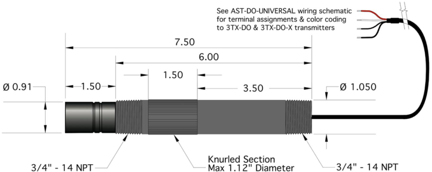
The AST-DO-UNIVERSAL-CONVERTIBLE configuration is suitable for inline, immersion or submersible type installations (see sections below for more details & specifics). Drawing above is shown with standard 1.50 inch insertion depth for inline use. Available up to 3.50 inch insertion depth as a special order option.
