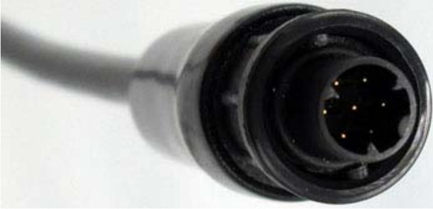
*Q7M sensor end of cable snap connector detail close-up view*
