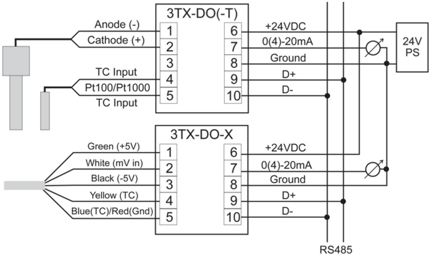
**Wiring Schematic Details for Without Pre-amplifier & with Integral Pre-amplifier Configurations of AST-D0-UNIVERSAL Galvanic Dissolved Oxygen Sensors with 3TX-D0(-X) Transmitters**
