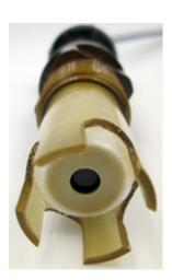
Simple to use industrial ion selective measurement systems are supplied complete with smart digital ISE sensor and mating field instrumentation ready for immediate commissioning in the field. Only a periodic grab sample offset calibration is required in the field. No standard solutions are required at all for commissioning nor for ongoing maintenance.
