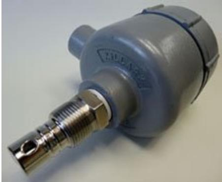
Industrial conductivity sensors for use up to 205 degrees Celsius and 500 psig suitable for measurements from 0.055 microSiemens and up to 2,000 milliSiemens. Applications supported include ultrapure water, strong acids, strong bases and concentrated electrolytes. Materials of construction include 316SS, Monel, Titanium, Hastelloy C-276 for electrodes and TEFLON, CPVC, KYNAR and PEEK for the insulator.
