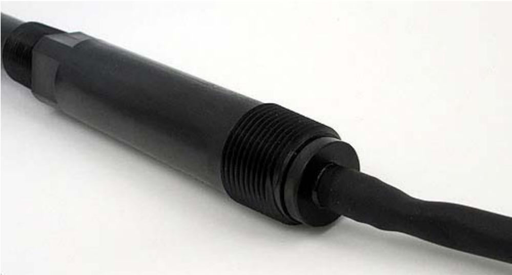
*Rear close-up of 6X61 analog sensor with WPIT polypropylene sealing & NORPRENE tubing installed; Fully submersible to 115 degrees Celsius Max*
