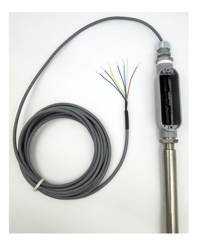
Integral bridge box installed on extension tube for easy quick disconnect sensor maintenance with Q7M/Q7F snap connector system for analog pH/ORP/ISE/D0 sensors with integral preamplifiers or HiQ4M/HiQ4F snap connector system for smart digital sensors (not shown)
