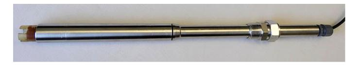
Details on just the 316SS sensor holder (on left) fitted with the short 12 inch extension tube (on right). These two parts fitted together constitute and insertion tube assembly. Also shown is the 5X31 series sensor (far left) as well as the 1"MNPT X 1.00"0.D. compression fitting and sealing cable glands. For use with the HOT-TAP valve retractable style the extension tube would be longer 36, 48 or 60 inch length as necessary for the given installation.
