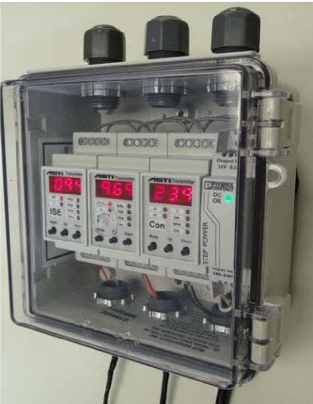
Triple Channel Nitrate, pH & Conductivity Transmitter
