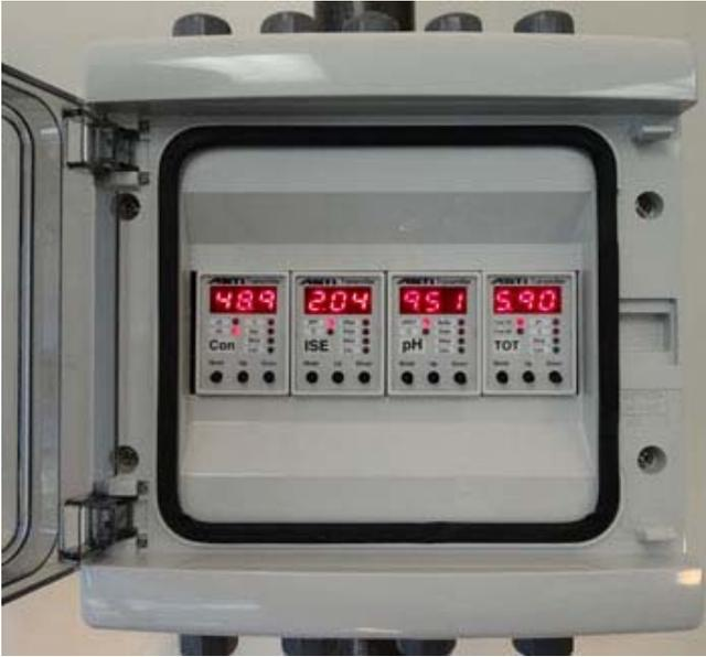
**Triple Channel Total Ammonia, pH & Conductivity Transmitter**
