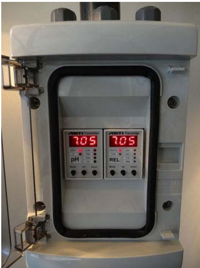
Single Channel pH Controller 3TX-2M-pH-A-REL
