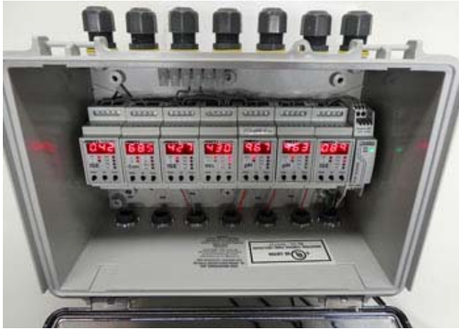
Seven Channel pH/ORP/ISE/Conductivity Assembly 3TX-7MF-ISE-CON-ISE-REL-pH-ORP-ISE-PS
