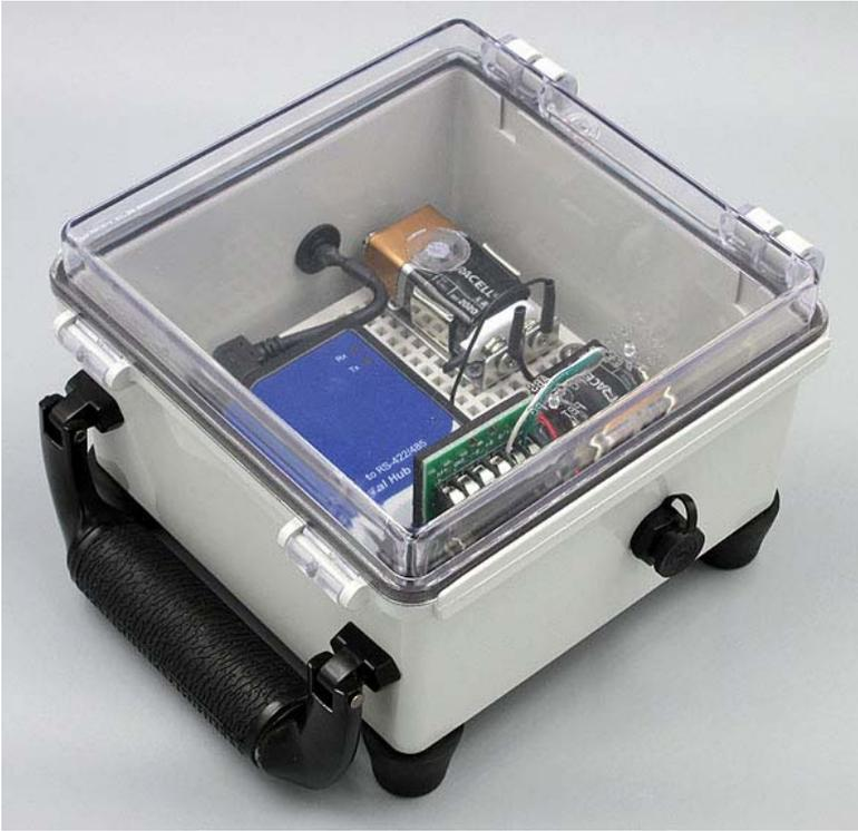
*Portable HiQ to Windows Bridge Box Close-Up detailing industrial RS-485 to USB converter.*
