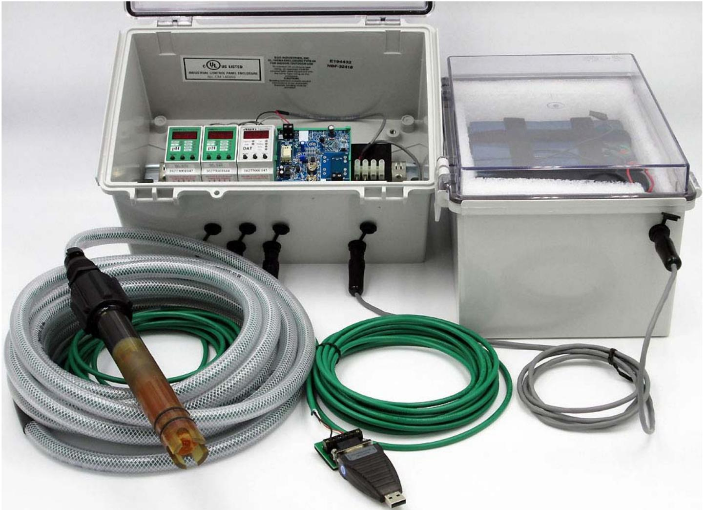
*Plug & Play Submersible pH & ORP Measurement System for Intermittent Battery-Powered Operation at Remote Installations detailed as [Case Study # 22](#)*
