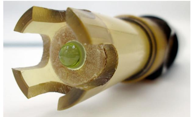
Close-up of ZEUS™ pH sensor measuring tip. Solid-state conductive polymer reference system (brown) is sealed to thick-wall break-resistant low-profile parabolic pH sensing element (green) protected by ultra-rugged 4 each protective tines for guard
