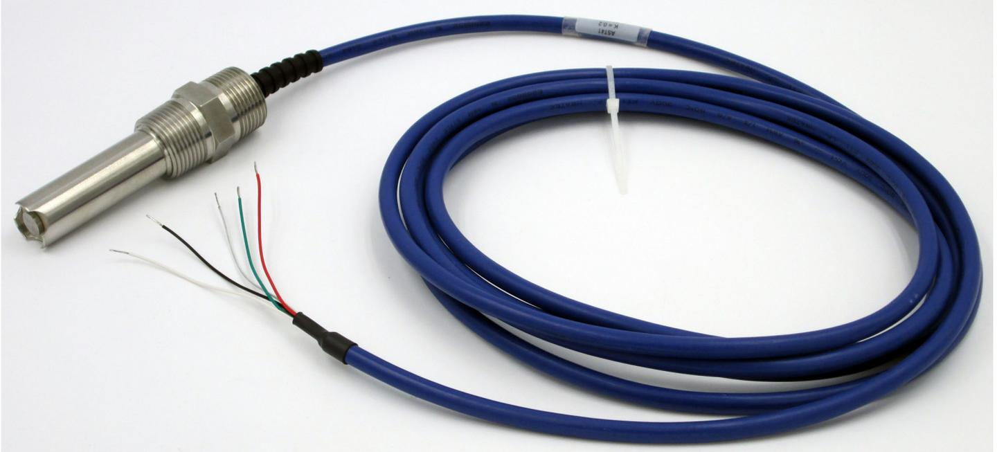
*The AST41 in the  $K=0.2/cm$  with extended insertion depth is an ideal choice for rugged submersible measurements especially when combined with the braid-reinforced blue cable option. The rear  $\frac{3}{4}$ " MNPT threads should be interfaced with a suitable immersion tube (a.k.a. standpipe) if the planned installation is submersible style.*
