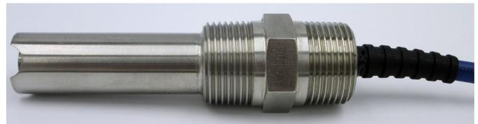
*Various close-up views of the AST41 in the  $K=0.2/cm$  with extended insertion depth in the without J-Box configuration. The open geometry can be ideal for situations of low-flow, high viscosity or else other potential fouling constituents that may be present in slurries and other abrasives in the solution. When used with the 3TX-CON transmitter this sensor can be used to measure up to 20,000  $\mu S/cm$  (20mS/cm) making it suitable for a wide range of potential applications.*
