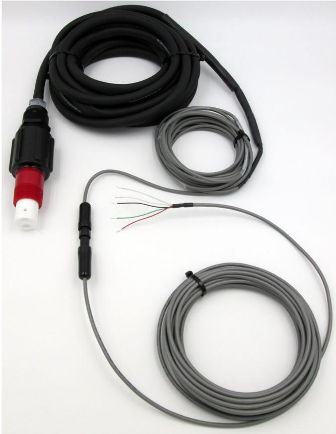
*AST60-HastC-2.0-1000-40-Q5M-WPB/20PP-VITON Submersible Contacting Conductivity K=2.0/cm Sensor with Hastelloy C-276 electrodes and VITON O-rings; 40 feet cable with Q5M snap connector; 20 feet NORPRENE hose installed*
