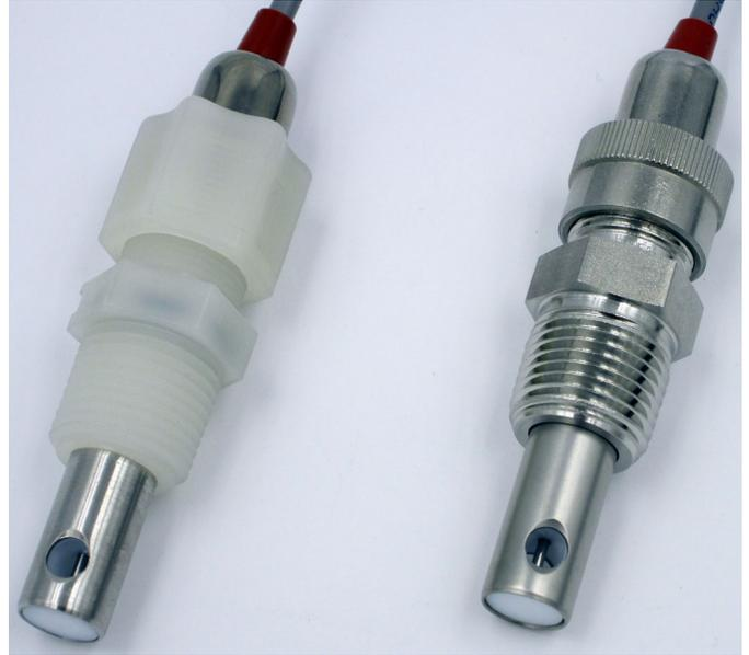
*AST51 sensors shown with 1/2" MNPT KYNAR (PVDF) and 316SS compression fittings both in the K=1.0/cm cell constant configuration from left to right, respectively. Wetted materials of construction 316SS (standard), titanium, Hastelloy C-276 for electrodes & EPDM (standard), Viton or Kalrez for elastomers. TEFLON (PTFE) is always the wetted insulator material.*
