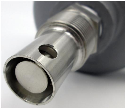
*Close-up of AST41 in K=0.05/cm cell constant. The K=0.1/cm cell constant is largely similar except for diameter & position of inner electrode.*
