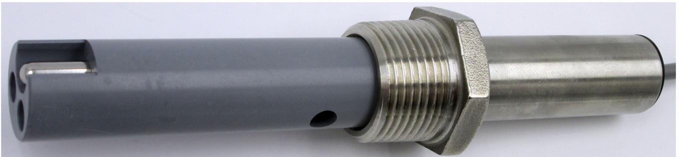
*The sensor shown above has 316SS electrodes and sensor body with CPVC insulator. The 316SS electrodes are not visible as they are located inside of the two bored holes that go along the length of the insulator and are purged by the two corresponding vent holes on each side. The exposed 316SS thermowell is, however, visible which provides for fast temperature measurement to ensure accurate conductivity values at any process condition.*
