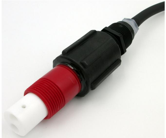
*Close-ups of waterproofing "B" sealing with NORPRENE tubing installed onto AST60 sensor in K=2.0/cm cell constant. Assembly is fully submersible without immersion tube.*
