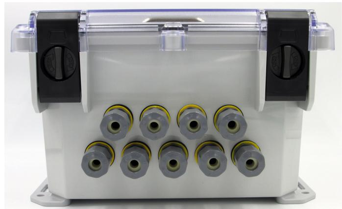
Top output side with latches have 9 each each 1/2" NPT cable glands factory installed giving a total of 14 each cable glands for the six channel controller (including 14 each sealing caps to cover all cable glands to ensure NEMA 4X rating of assembly when no cables are installed). When ethernet cable is used install the alternate cable gland provided (not shown above).
