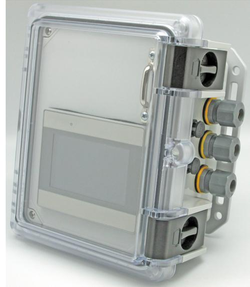
Two (2) channel controller with 4.3" Touchscreen shown on left with output ports & on right with input ports. Two HiQ4FP panel connectors are NEMA 6P input ports for HiQDT sensors. Integral 1/2"NPT cable glands number three on right input side & four on left output side. NEMA 4X wiring of power, analog & digital outputs, relays & remote access via ethernet port with oversize gland.
