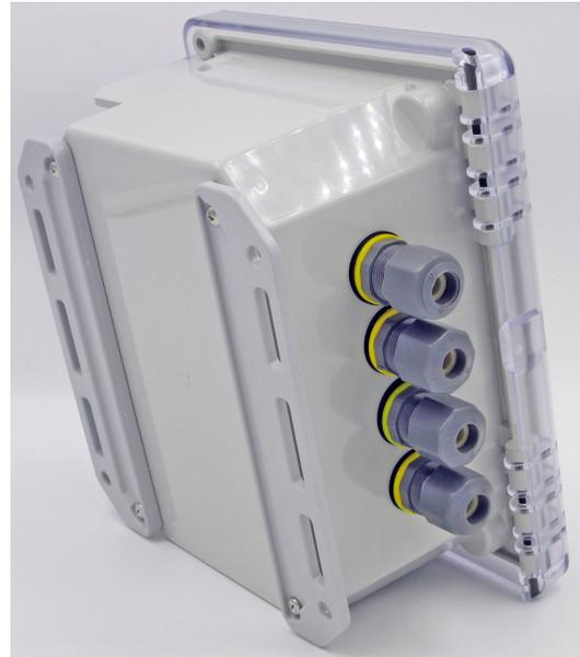
*The rear mounting plates on back of the controller make it ready for immediate wall or pipe mounting in field without purchase of any additional specialized hardware. Standard commercial U-Bolt can achieve a pipe mounting scheme & commercial bolts and washers can be used to achieve mounting to a wall or plate. Inquire for any planned installation schemes that are not covered by the brackets shown above which are suitable for most all of the typical wall or pipe mounting schemes.*
