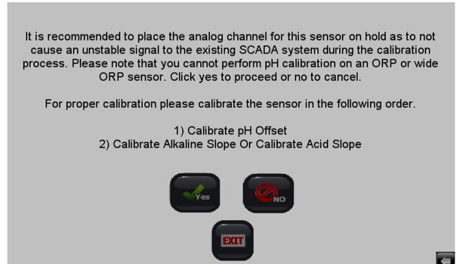
It is recommended to place the analog channel for this sensor on hold as to not cause an unstable signal to the existing SCADA system during the calibration process. Please note that you cannot perform pH calibration on an ORP or wide ORP sensor. Click yes to proceed or no to cancel.
