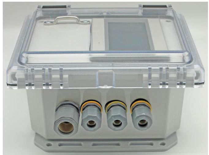
*Left output side has 3 each standard 1/2" NPT cable glands and 1 each oversized gland for ethernet network cable factory installed giving a total of 7 each cable glands for the two channel controller (7 each sealing caps included to cover glands when no cables installed). When ethernet cable is not used then swap oversized gland with provided spare standard cable gland.*
