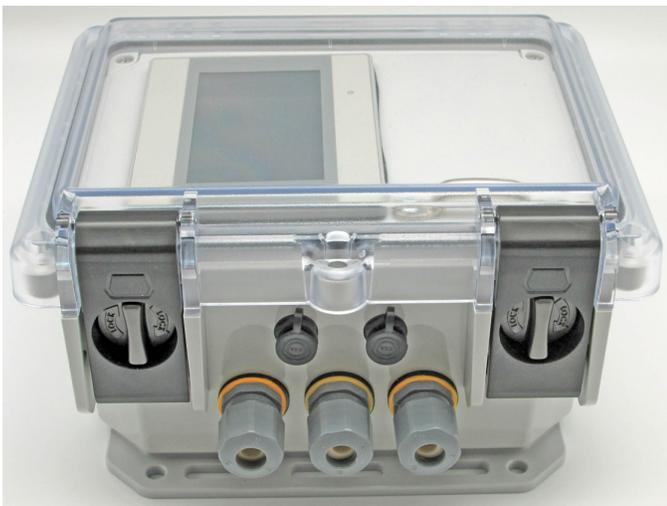
*On right input side are factory installed 3 each 1/2" NPT cable glands and 2 each NEMA 6P rated female snap panel mount connectors for plug & play hot-swappable HiQDT smart digital sensors. Sealing cap for panel connectors should be secured and provided caps for cable glands affixed when not in use to maintain the integrity of the NEMA 4X assembly rating.*
