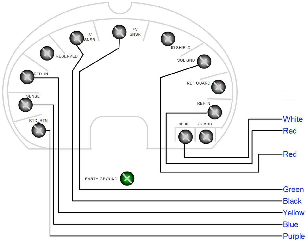
**Note 1: Temperature element (RTD) is Platinum 1000 Ohm type unless otherwise specified.**
