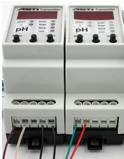
Input terminals close-up of PtD sensor to 2 ea 3TX-pH
