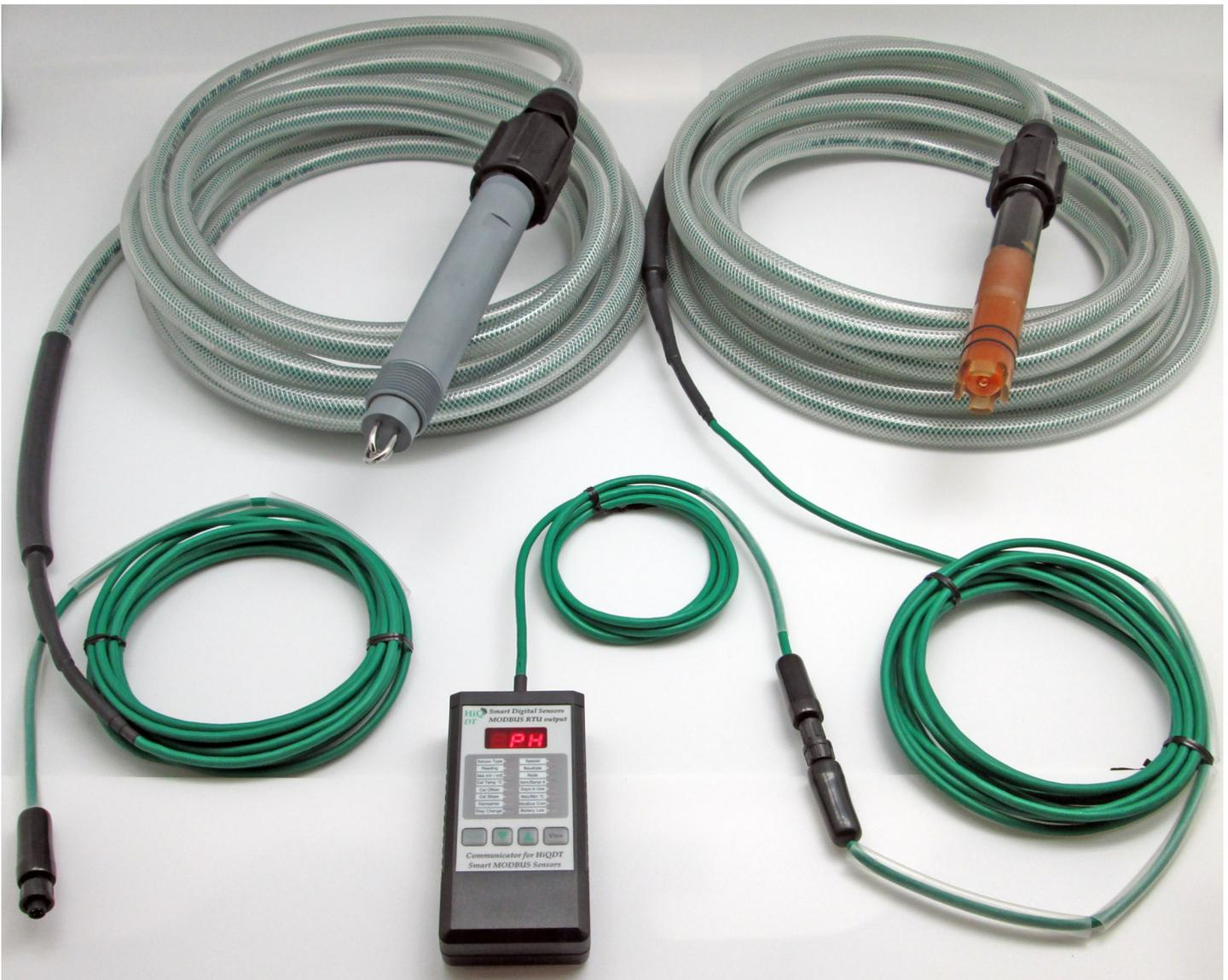
Since these are smart digital sensors can be pre-calibrated at any location of convenience and hot-swap plug and play exchanged in the field with the NEMA 6P rated waterproof connectors. This means that no special training at all is required for the swap-out of ASTI smart digital pH, ORP & conductivity sensors in the field.
