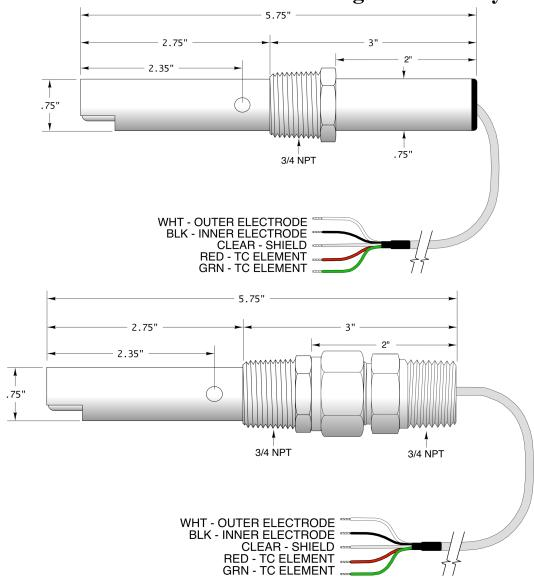
Drawings of AST52 cell constant configurations shown without waterproofing option. Please inquire to factory for overall sensor length and dimensional details is a waterproofing option is to be added to sensor. The compression fitting style assembly can also be used for fully submersible so long as a suitable immersion rod (a.k.a. standpipe) is secured to the rear ¾"MNPT threads.
