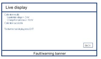
Repeat this Standardize (grab) calibration as often as may be required to account for sensor drift over time for the given installation. The frequency with which this procedure is performed will vary from site to site depending upon a number of factors.
