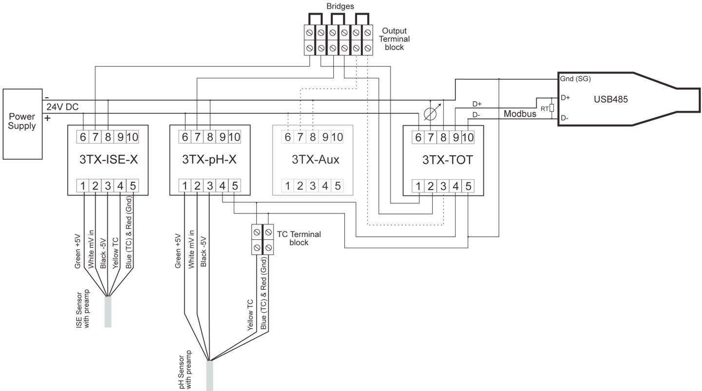
**Note 1:** The 3TX-pH transmitter can be used for either pH or ORP measurement and wiring connections are the same for both pH and ORP sensors (only the Parameter No. 03 needs to be changed/toggled to select between the two input types). For ORP sensors select mV as the input type in P03.
