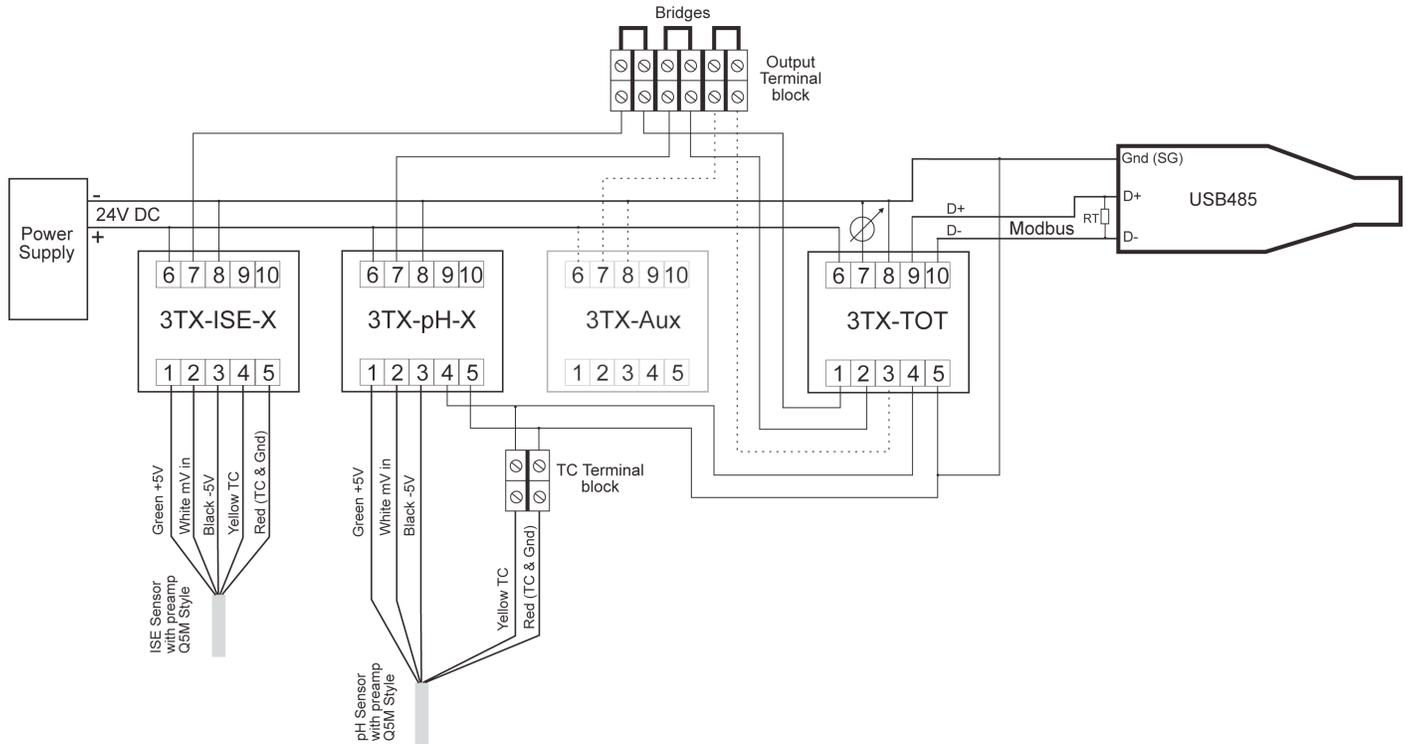
\* The second side of TC is tied together with the common/reference signal inside the sensor when the Q5M & Q5F connector are used and so only the red wire need to wired to terminal 5.
