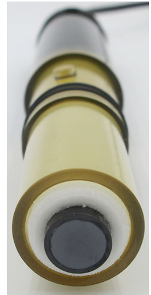
* Solid-state ion selective sensor with large surface industrial sensing element
