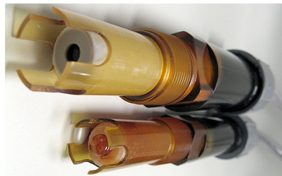
Typical Immersion Style Fluoride Ion Selective & High HF Resistant pH Sensor for use in acid etching processes and fluoride wastewater treatment (WWT) plants. Both fluoride ISE & pH sensors required to continuously measure total fluoride species.
