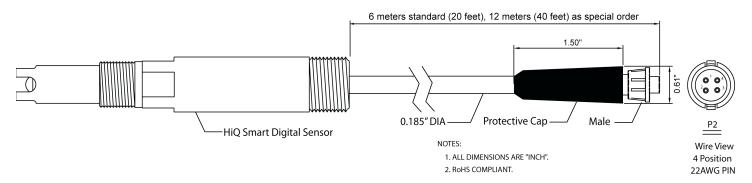
Detail drawing for female snap to male snap HiQ4F-Xm-HiQ4M cable extensions:
