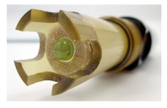
Close-up of ZEUS<sup>™</sup> pH sensor measuring tip. Solid-state conductive polymer reference system (brown) is sealed to thick-wall break-resistant low-profile parabolic pH sensing element (green) protected by ultra-rugged 4 each protective tines for guard
