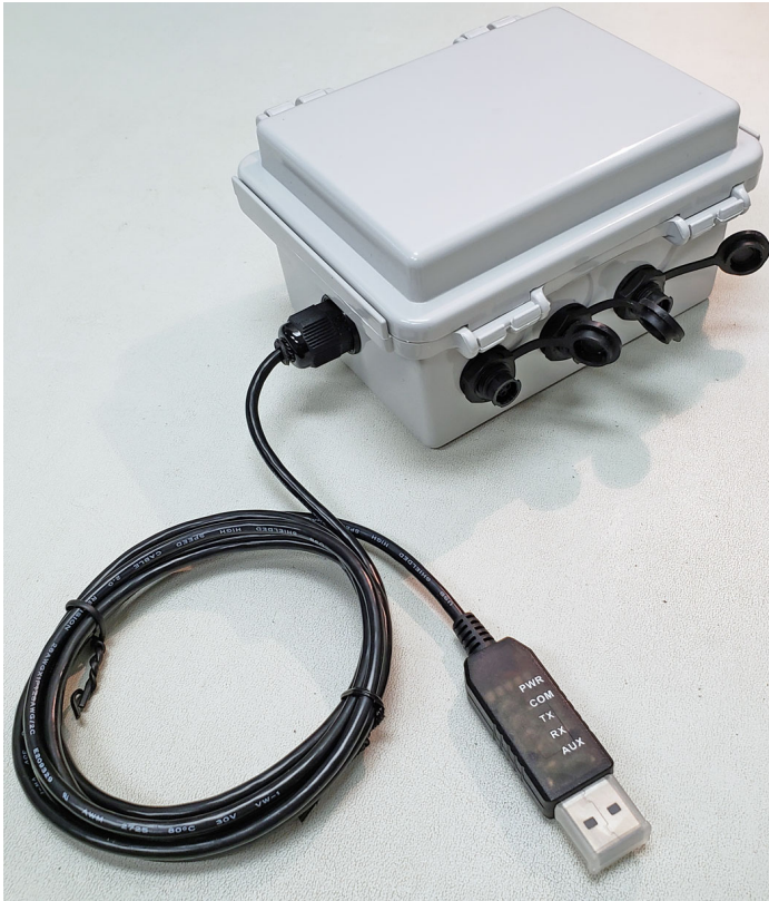
Integral 1.5 meter (5 foot) USB cable provides power to energize sensors as well as all communications between Windows Software acting as RS485 MODBUS RTU master and Smart Sensors acting as slaves
