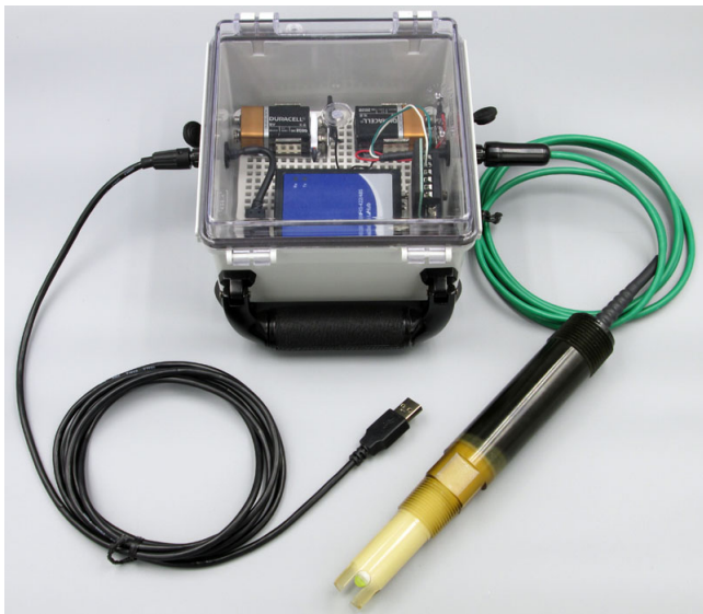
Digital Sensor & USB Cable Connected with Portability Package Option
