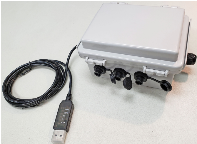
Up to 3 each smart sensors can be interfaced using HiQ4FP female panel mount connectors with male HiQ4M sensor cable end termination. The sensor connections are NEMA 6P rated when interfaced. The cap should be affixed when not in use to maintain the waterproof rating. The 1/4" MNPT cable gland on right can be used to an additional cable to send communications or power from or two an external device.
