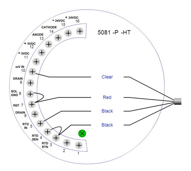
Note 1: Temperature element (RTD) is Platinum 1000 Ohm type unless otherwise specified.
