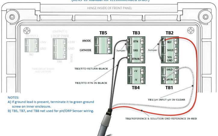
Note 1: Temperature element (RTD) is Platinum 1000 Ohm type unless otherwise specified.
