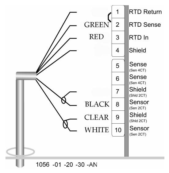
Note 1: The temperature compensation element is 1000 Ohm Platinum.
