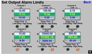
High & Low relay setpoints for process value from each channel with time delay.
