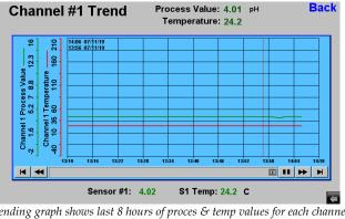
Trending graph shows last 8 hours of proces & temp values for each channel. Unlimited datalogging capacity w/ 32GB storage, remotely accessible via FTP.
