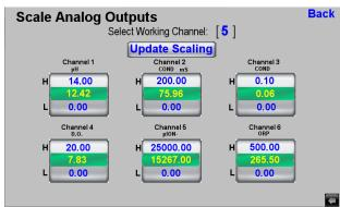
Each analog output fully scalable in engineered units. For EC sensors units available are mS/uS or PSU or TDS or else MegaOhm (MQ) resistivity.
