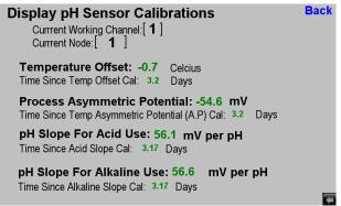
Sensor calibrations for each channel are displayed & datalogged including time since each calibration was last performed to facilitate best practice maintenance.
