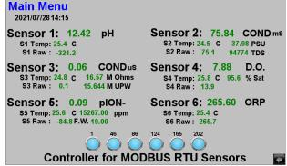
Main display for the six channel controller. Other screens is obtained through the main menu. Status updates, alarms & alerts are scrolled across top of screen.
