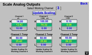
Each temperature output channel is associated with a specific sensor input channel and scaled as desired along with the process value for that sensor.
