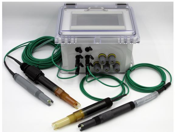
*Six (6) channel HiQDT-CTRL-6CH controller shown with 4 each smart RS485 MODBUS RTU pH sensors connected (two top ports are unused). Controller is NEMA 4X when the door is latched. Hot swappable sensors with plug & play snap connectors are NEMA 6P rated when interfaced. The 3 & 6 channel controllers with 7.0" touchscreen are available in configurations that are suitable for hazarduous Class I, Division II locations.*
