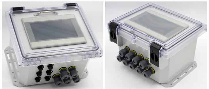
Clear hinged latched door provides outstanding protection for advanced touchscreen HMI from environment as part of NEMA 4X rated assembly. To access internal components of controller simply remove two top screws & open with pull handle. One left are 6 each NEMA 6P rated female snap panel mount connectors for plug & play smart digital sensors and 5 each cable glands while on right are 9 each cable glands (all factory installed).
