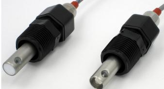
AST51 sensors shown with  $\frac{3}{4}$ " MNPT polypropylene (PP) compression fittings in the K=1.0/cm & K=0.1/cm cell constant configurations from left to right, respectively.
