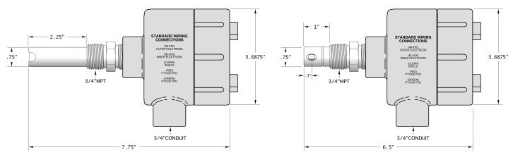
NOTE 1: The AST41 sensor can be supplied with ASTI supplied cable or else customer supplied cable can be used and connected to the terminals in the J-Box. NOTE 2: The AST41 sensors can be supplied without J-Box if customer shall supply and install their own. Contact factory for assistance if you wish to use this scheme.
