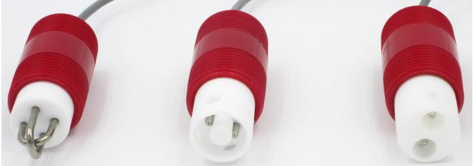
AST60 contacting conductivity sensors shown in K=0.1, 1.0 and 2.0 cell constants from left to right, respectively.
