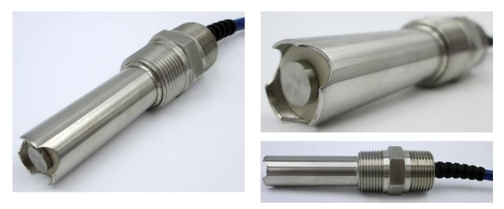
Various close-up views of the AST41 in the K=0.2/cm with extended insertion depth in the without J-Box configuration. The open geometry can be ideal for situations of low-flow, high viscosity or else other potential fouling constituents that may be present in slurries and other abrasives in the solution. When used with the 3TX-CON transmitter this sensor can be used to measure up to 20,000  $\mu$ S/cm (20mS/cm) making it suitable for a wide range of potential applications.
