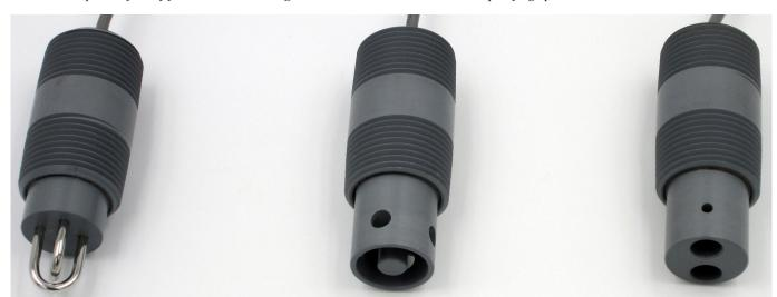
AST50 contacting conductivity sensors shown in K=0.1, 1.0 and 2.0 cell constants from left to right, respectively.
