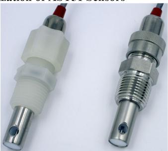
AST51 sensors shown with ½" MNPT KYNAR (PVDF) and 316SS compression fittings both in the K=1.0/cm cell constant configuration from left to right, respectively. Wetted materials of construction 316SS (standard), titanium, Hastelloy C-276 for electrodes & EPDM (standard), Viton or Kalrez for elastomers. TEFLON (PTFE) is always the wetted insulator material.
