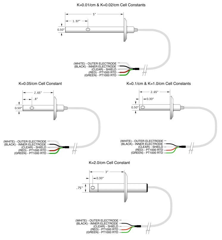
The flanges for the K=0.01/cm, K=0.02/cm, K=0.05/cm, K=0.1/cm & K=1.0/cm sanitary conductivity sensors are shown with a 1.5" TRI-CLOVER flange. The K=2.0/cm sanitary conductivity sensor is shown with a 2" TRI-CLOVE flange. The smallest TRI-CLOVER flange for K=2.0/cm sensor is the 1.5" where all sizes are available for all other cell constants. All dimension in inches.
