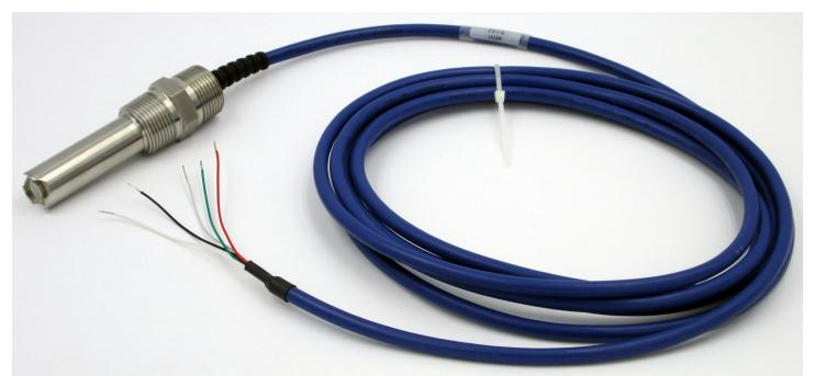
The AST41 in the K=0.2/cm with extended insertion depth is an ideal choice for rugged submersible measurements especially when combined with the braid-reinforced blue cable option. The rear  $\frac{3}{4}$ " MNPT threads should be interfaced with a suitable immersion tube (a.k.a. standpipe) if the planned installation is submersible style.
