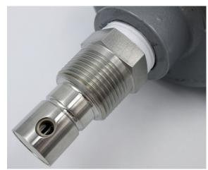
Close-up of AST41 in K=2.0/cm cell constant. The K=1.0/cm cell constant is largely similar except for diameter of inner electrode & diameter of vent hole.
