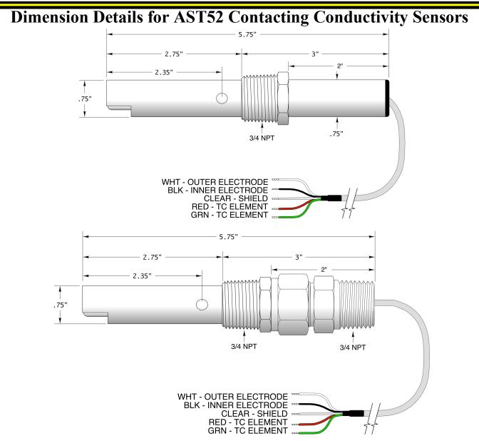
Drawings of AST52 cell constant configurations shown without waterproofing option. Please inquire to factory for overall sensor length and dimensional details is a waterproofing option is to be added to sensor. The compression fitting style assembly can also be used for fully submersible so long as a suitable immersion rod (a.k.a. standpipe) is secured to the rear  $\frac{3}{4}$ "MNPT threads.
