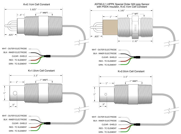
Drawings of AST50 and AST60 in the available K=0.1/cm, K=1.0/cm and K=2.0/cm cell constant configurations are shown without waterproofing option. Please inquire to factory for overall sensor length and dimensional details is a waterproofing option is to be added to sensor.
