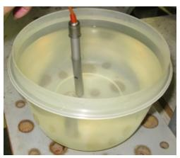
3. WIPE ELECTRODE AREAS WITH ACETONE USING PIPE CLEANERS AND COTTON TIPPED SWABS.
