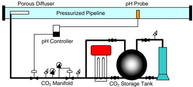
When pH control is critical to your process or effluent quality, CO<sub>2</sub> can be a most viable alternative.
