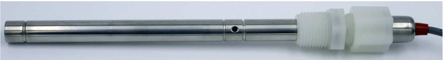
AST10 Contacting Conductivity Sensor in K=10.0/cm cell constant with Hastelloy C-276 & Viton Wetted Materials & KYNAR fitting
