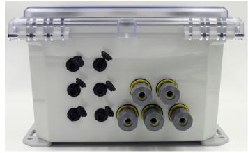
On bottom input side are factory installed 5 each ½" NPT cable glands and 6 each NEMA 6P rated female snap panel mount connectors for plug & play hot-swappable HiQDT smart digital sensors. Sealing caps for panel connectors & cable glands must be secured when not used to maintain NEMA 4X rating. Three (3) panel connector unused in the 3 channel configuration.
