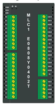
Contact Relays for PROCESS High & Low Setpoints for Channels 1, 2, 3 on MLC1-E0808Y0402T
