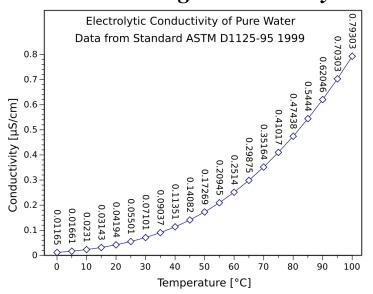
The conductivity of pure water varies significantly with temperature in a well-defined but non-linear fashion as detailed in the graph to left. This behavior is preprogrammed into the HiQDT-CON-L MODBUS RTU conductivity sensors for the automatic temperature compensation feature to make it suitable for ultrapure water (UPW) type applications.
