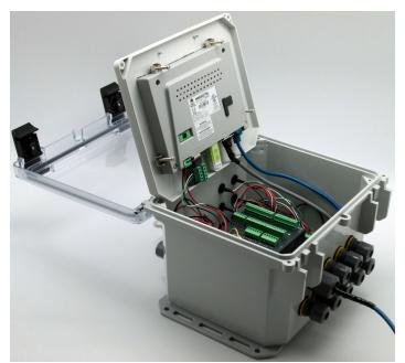
HiQDT-CTRL-6CH six (6) channel controller with 7.0" touchscreen HMI is shown with lid & swivel plate open. The HMI & PLC are interfaced with only the power terminal block and communication cable cable allowing for simple and convenient replacement if damaged. Clear hinged latched door provides NEMA 4X protection for advanced touchscreen HMI from environment. To access internal components of controller simply remove two top screws & open with pull handle.
