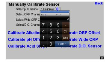
The usual caveats apply before performing calibration on you dissolved oxygen (D.O.) sensor. The channel that will be calibrated should be placed on hold prior to performing the calibration especially if the values obtained from the sensor are used for any type of realtime closed loop control purposes.
