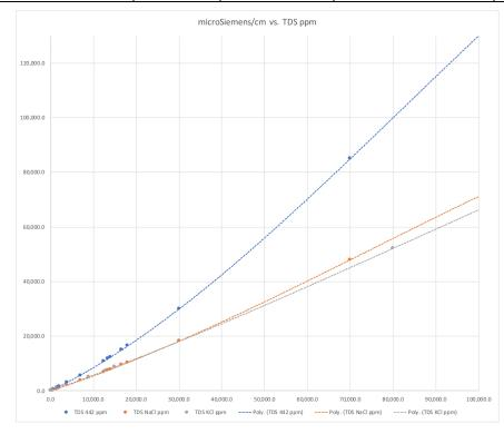
Total dissolved solids (TDS) units are computed from measured conductivity. The curves that define relationship between the measured conductivity and user selectable total dissolved solid (TDS) units of NaCl, KCl or 442 are preprogrammed into sensor with full range of 0 to 100,000 ppm. The actual usable range may be limited by the choice of cell constant and range mode in which the sensor is operated.
