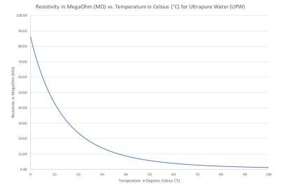
Graph above shows relationship between the resistivity of pure water at various temperatures. Computed resistivity MegaOhm ( $M\Omega$ ) units are the inverse of measured conductivity and so are the mirror image of the conductivity at various temperatures for ultrapure water (UPW). Graph above shows absolute raw resistivity at various temperatures. Resistivity values sent include ATC referencing reading to 25 °C state.
