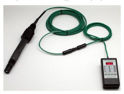
The handheld communicator (HHC) can both search for the node of the connected sensor as well as to modify the node if desired. Using this battery powered handheld communicator (HHC) to control the node assignments of the MODBUS RTU sensors allows for a very convenient field installation scheme for the commissioning of the advanced touchscreen controllers.
