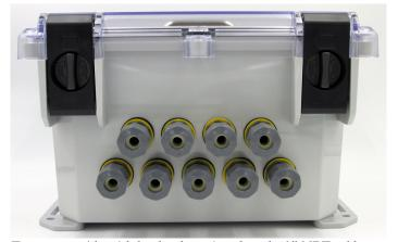
Top output side with latches have 9 each each ½" NPT cable glands factory installed giving a total of 14 each cable glands for the six channel controller (including 14 each sealing caps to cover all cable glands to ensure NEMA 4X rating of assembly when no cables are installed). When ethernet cable is used install the alternate cable gland provided (not shown above).
