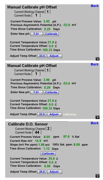
It is recommended to place the analog channel for this sensor on hold as to not cause an unstable signal to the existing SCADA system during the calibration process. Please note that you cannot perform pH calibration on an ORP or wide ORP sensor. Click yes to proceed or no to cancel.
