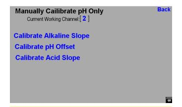
You must first perform A pH offset calibration before you can perform a slope calibration.
