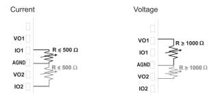
Channel #1 → Voltage 0-10VDC Sent between AGND & V01
