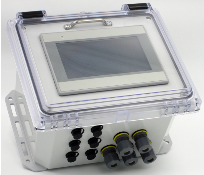
Six (6) channel controller with 7.0" touchscreen shown on left with bottom input ports & top output ports shown on right. Six (6) HiQ4FP panel connectors are waterproof input ports for sensors. Integral 1/2"NPT cable glands number five (5) on bottom input side & nine (9) on output side for NEMA 4X wiring of power, analog & digital outputs, contact relays & remote access via ethernet port.
