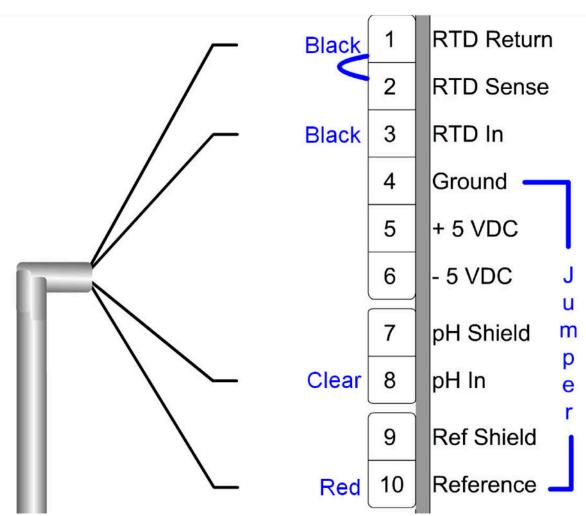
Connection from Iotron<sup>TM</sup> Sensor to Terminal Block in Rosemount Transmitter
