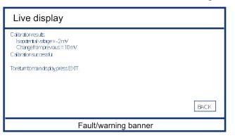
9. Repeat this Standardize (grab) calibration as often as may be required to account for sensor drift over time for the given installation. The frequency with which this procedure is performed will vary from site to site depending upon a number of factors.
