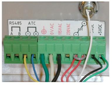
Note 1: Temperature Compensator is either a 3000 Ohm Balco or 1000 Ohm Platinum Element. You must set this TC Value in the Calibration Mode (if not preconfigured). Use Code: **rES** for the AtC setting if a 3000 Ohm Balco Resistor is present or use Code: **Pt** for the AtC setting if a 1000 Ohm Platinum Element is present
