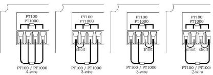
Special hook-up schematics of 2-wire and 3-wire PT100 or PT100 temperature compensation (TC) elements to 2TX.
