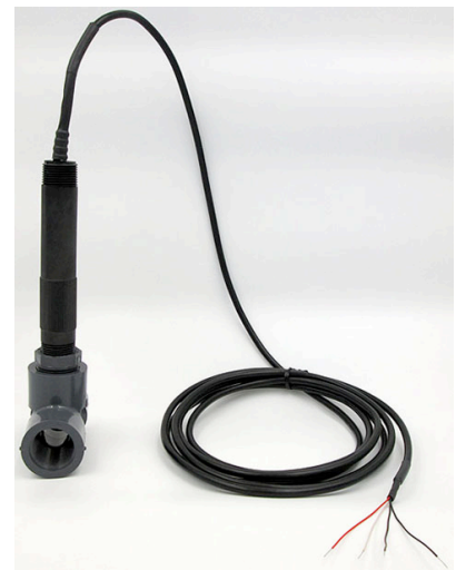
AST-DO-UNIVERSAL dissolved oxygen convertible style galvanic DO sensor shown threaded into tee with front 3/4" MNPT threads for inline use. Alternate inline installation uses 1" MNPT twist lock quick disconnect bayonet style sensor with mating receptacle to allow for fast and simple removal & installation from process without damaging the cable due to coiling from repeated use over time that can occur with screw-in type inline installations.
